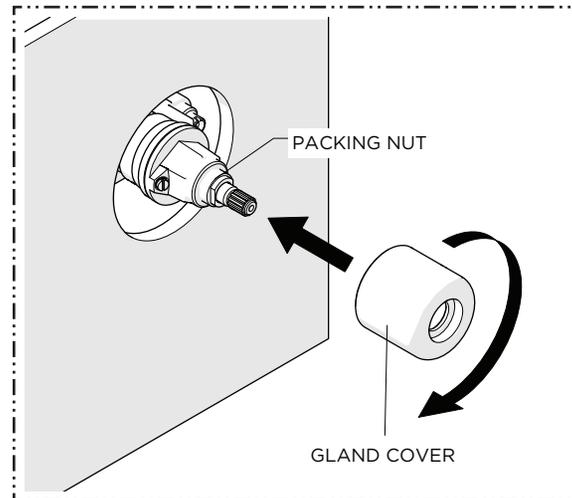
10. Thread and securely tighten the GLAND COVER onto the PACKING NUT.
