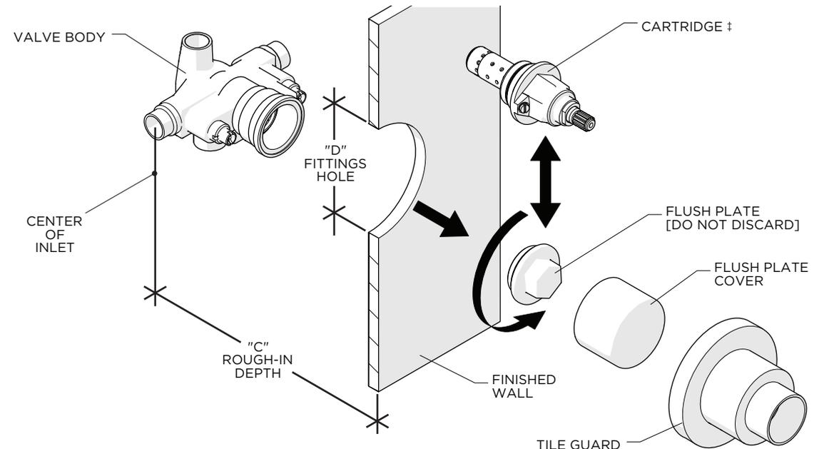
‡ **IMPORTANT:** The PRESSURE BALANCE CARTRIDGE, is packaged separately and provided with the VALVE. SET ASIDE UNTIL FINAL TRIM INSTALLATION!
