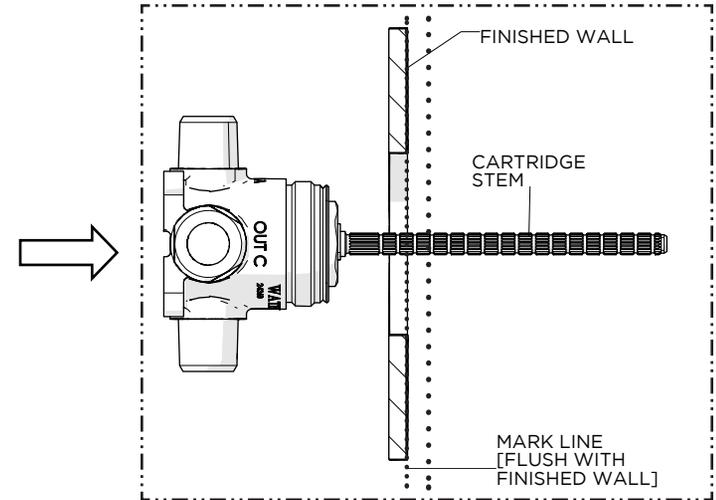
3. Mark the CARTRIDGE STEM where it protrudes past the finished wall.
