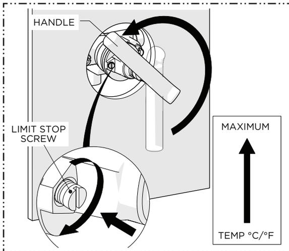
9. Open the VALVE to the **maximum** desired bathing temperature verified with a thermometer then turn the LIMIT STOP SCREW clockwise until it seats.
