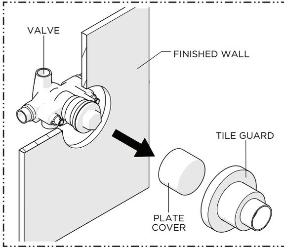
1. Remove the TILE GUARD and PLATE COVER from the VALVE when the TRIM is ready to be installed.
