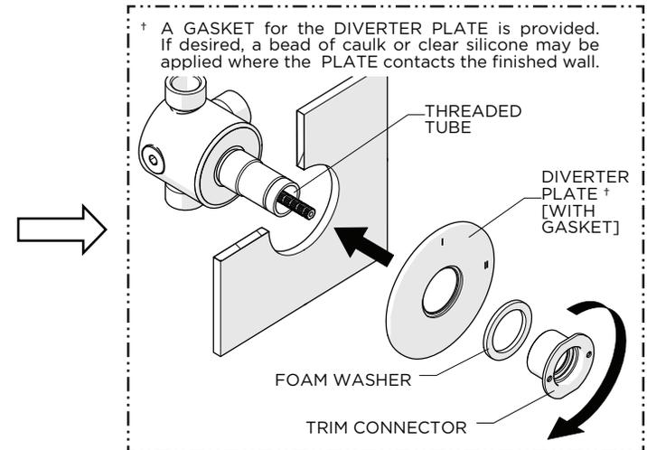
† A GASKET for the DIVERTER PLATE is provided. If desired, a bead of caulk or clear silicone may be applied where the PLATE contacts the finished wall.
