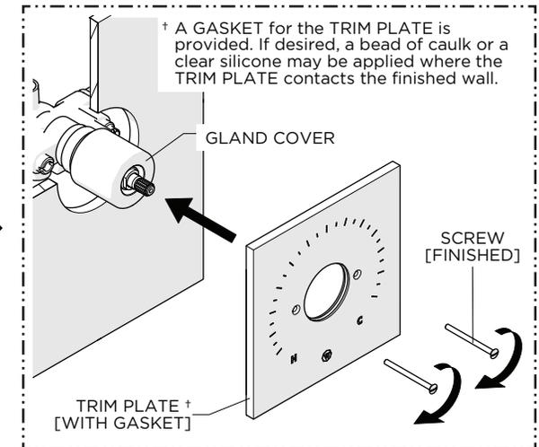
11. Slide the TRIM PLATE † [WITH GASKET] over the GLAND COVER then thread and securely tighten the SCREWS.
