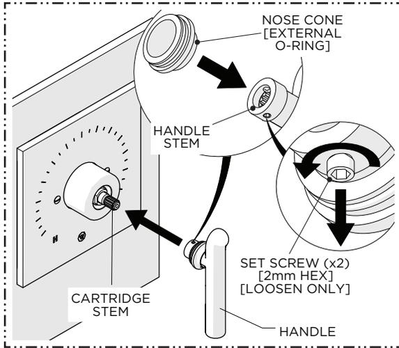
12. Slide the NOSE CONE over the HANDLE STEM then loosen the SET SCREWS (x2) and attach the HANDLE to the CARTRIDGE STEM.
