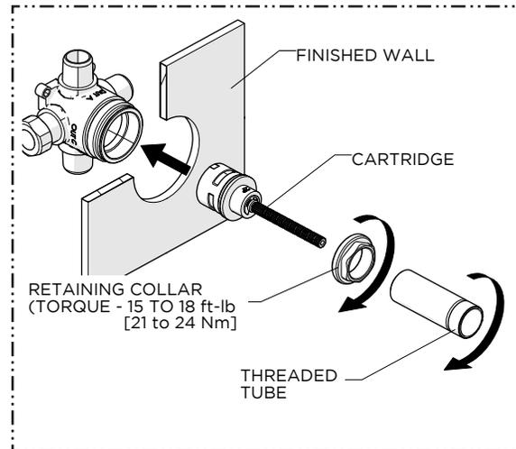
5. Thread the THREADED TUBE back onto the CARTRIDGE until snug.
