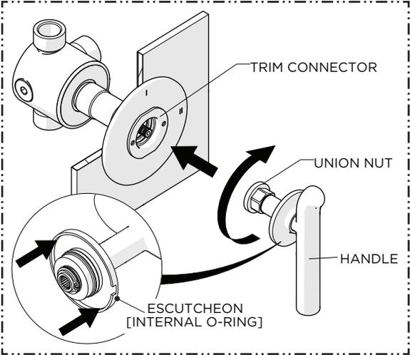
7. **CAREFULLY** slide the ESCUTCHEON up the HANDLE to expose the UNION NUT then, with the HANDLE in the desired orientation, thread the NUT into the TRIM CONNECTOR until snug.
