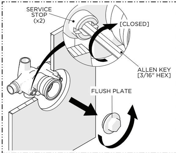
3. After the lines have been fully flushed, **CLOSE** the SERVICE STOPS (hot & cold) then unthread and remove the FLUSH PLATE.
