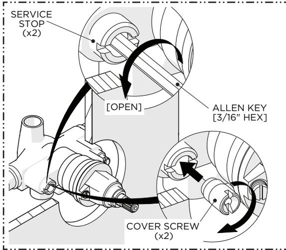
6. **OPEN** the SERVICE STOPS (hot & cold) then re-install the COVER SCREWS (x2).
