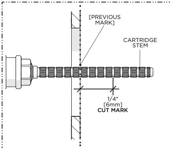
4. Carefully cut the CARTRIDGE STEM 1/4" [6mm] in front of the previous mark so the STEM will protrude 1/4" [6mm] from the finished wall surface.
