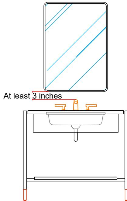
Choose your installation location to allow ample clearance to open the cabinet door. Allow at least 3 inches of clearance above or below the cabinet door for lighting and faucet clearance.
