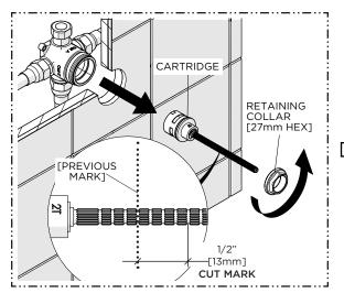
Unthread the RETAINING COLLAR and remove the CARTRIDGE then cut the CARTRIDGE STEM 1/2" [13mm] in front of the previous mark so the STEM will protrude 1/2" [13mm] from the finished wall surface.
