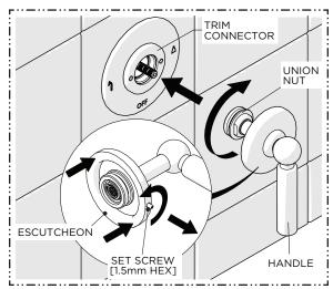
Loosen [do NOT remove] the SET SCREW at the base of the ESCUTCHEON then CAREFULLY slide the ESCUTCHEON up the HANDLE to expose the UNION NUT
