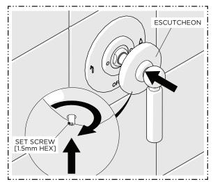
8. CAREFULLY slide the ESCUTCHEON down the HANDLE to conceal the TRIM CONNECTOR, then thread the SET SCREW to secure the position of the ESCUTCHEON.
