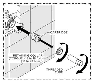
Re-insert the CARTRIDGE into the VALVE then thread and securely tighten the RETAINING COLLAR to the specified torque setting shown.
