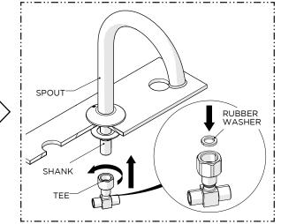
Thread and securely tighten the TEE onto the SHANK making sure to use the RUBBER WASHER provided.
