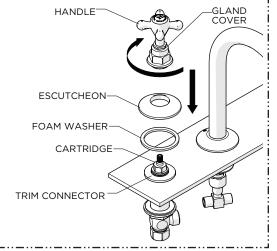
6. Making sure the FOAM WASHER is beneath the ESCUTCHEON, place the ESCUTCHEON over the TRIM CONNECTOR then insert the GLAND COVER into the ESCUTCHEON and thread it onto the CARTRIDGE until it stops.
