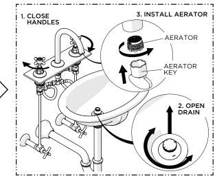
17. Close the HANDLES, open the DRAIN to drain the water, and re-install the AERATOR.
