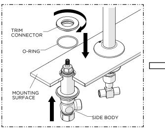
5. Insert the SIDEBODY through the hole on the mounting surface from below then, using the O-RING provided, thread the TRIM CONNECTOR back onto the SIDEBODY until it stops and let it rest on the mounting surface.
