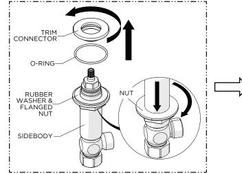
4. Unthread and remove the TRIM CONNECTOR from the SIDEBODY then fully thread the NUT down the SIDEBODY.
