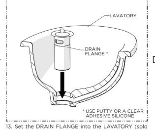
3. Set the DRAIN FLANGE into the LAVATORY (sold separately) using putty or a clear silicone.
