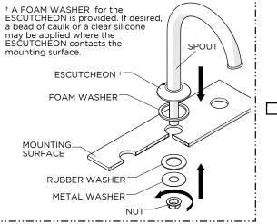
2. Insert the SHANK through the hole on the mounting surface, making sure the FOAM WASHER is beneath the ESCUTCHEON, then re-install the LOWER DECK WASHERS and securely tighten the NUT.
