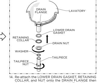
COLLAR, and NUT onto the DRAIN FLANGE then thread and securely tighten the NUT, making sure the GASKET makes a full seal on the underside of the LAVATORY, and re-attach the TAILPIECE using the WASHER and NUT provided.
