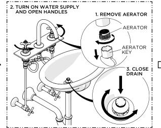
16. Remove the AERATOR, turn on the water supply and open the HANDLES to flush out the supply lines, and inspect all the connections for leaks then close the DRAIN to ensure it functions properly.
