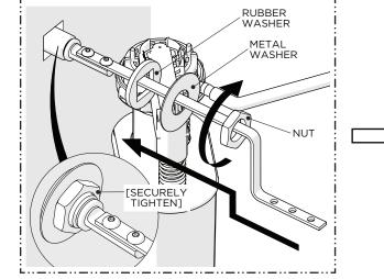
3. Re-install the RUBBER WASHER, METAL WASHER, and RETAINING NUT making sure to securely tighten the NUT.
