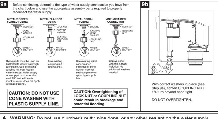
▲ WARNING: Do not use plumber's putty, pipe dope, or any other sealant on the water supply connection to this tank. If the connection leaks after hand tightening, replace the supply line. If the connection continues to leak with the new supply line, replace the fill valve.
