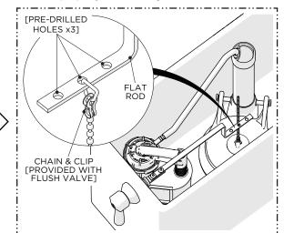
Using the CLIP provided with the FLUSH VALVE, connect the PULL CHAIN to one of the holes on the FLAT ROD. Adjust the CHAIN length and/or its position on the FLAT ROD to ensure the FLUSH VALVE is lifted when the HANDLE is rotated.
