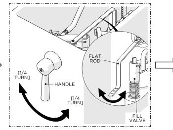
4. Rotate the HANDLE forwards and backwards to ensure the ROD rotates freely and is not obstructed by anything include the FILL VALVE.
