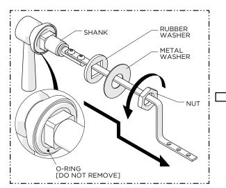
1. Remove the RETAINING NUT, METAL WASHER, and RUBBER WASHER from the FLUSH LEVER SHANK.
