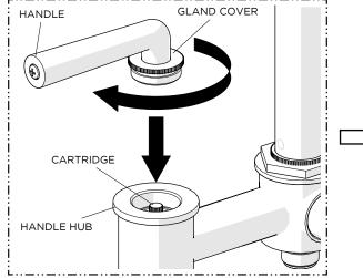
7. With the HANDLE held in the desired orientation, thread the GLAND COVER into the HANDLE HUB until snug.
