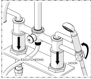
Rotate the HOOK to the desired position then slide the ESCUTCHEONS down until they contact the mounting surface.
