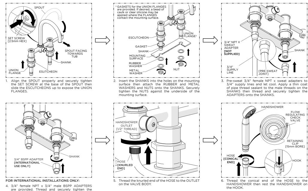
**NOTE:** A FLOW REGULATING CHECK VALVE is located inside the inlet of the HANDSHOWER.
