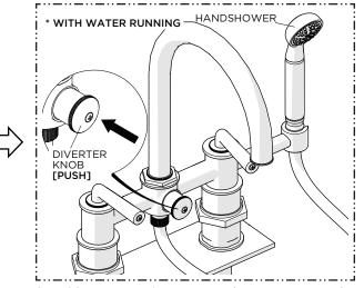
With water running, operate the DIVERTER KNOB to ensure it and the HANDSHOWER function properly.
