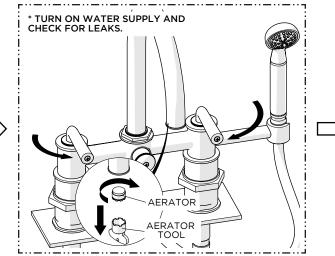
8. Remove the AERATOR using the TOOL provided then turn on the water supply and operate the HANDLES to flush out the supply lines and check all connections for leaks.
