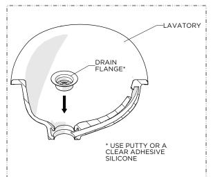
14. Set the DRAIN FLANGE in the LAVATORY (sold separately) using putty or a clear adhesive silicone.
