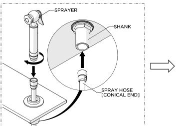
13. Insert the SPRAY HOSE [conical end] through the SHANK and the ESCUTHCHEON then thread and securely tighten the SPARYER onto the HOSE.
