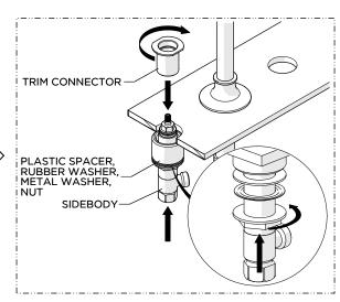
Thread the TRIM CONNECTOR onto the SIDEBODY until it stops and let it rest on the mounting surface then hand-tighten the NUT against the underside of the mounting surface.
