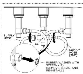
17. Turn off the water and unthread both the SUPPLY HOSES from the TEE to remove and clean the RUBBER WASHERS WITH SCREENS then re-install the WASHERS and HOSES.
