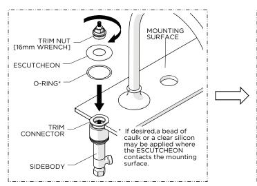
7. Place the ESCUTCHEON and O-RING over the TRIM CONNECTOR then thread and securely tighten the TRIM NUT into the TRIM CONNECTOR.
