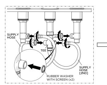
10. Connect the SIDEBODIES to the TEE using the SUPPLY HOSES provided. Securely tighten the HOSES and ensure they are not pinched/kinked.
