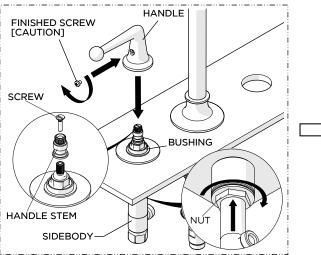
Place the HANDLE onto the HANDLE STEM, thread and securely tighten the FINISHED SCREW, ensure the HANDLE is in the desired orientation then securely tighten the NUT on the SIDEBODY.
