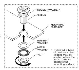
12. Insert the SHANK through the hole on the mounting surface making sure the RUBBER WASHER provided is beneath the ESCUTCHEON then re-install the WASHERS then securely tighten the NUT.
