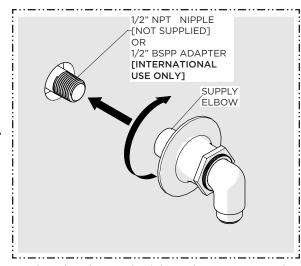
Thread and securely tighten the SUPPLY ELBOW onto the NPT NIPPLE or BSPP ADAPTER.
