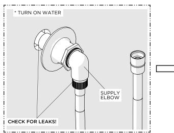
Turn on the water and a diverter/wall valve (sold separately) to flush out any debris in the supply line and inspect all connections for leaks then turn the water off.
