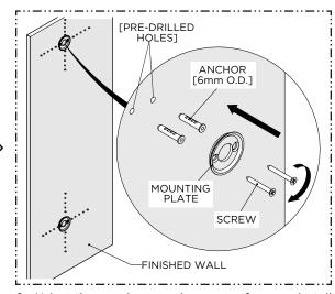
Using the previous marks as a reference, install the MOUNTING PLATES using the ANCHORS, if necessary, and SCREWS provided.
