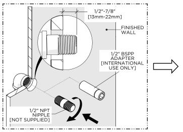
Install a 1/2" NPT NIPPLE (not supplied) and ensure it protrudes 1/2"- 7/8" [13mm - 22mm] from the finished wall.
