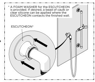
Slide the ESCUTCHEON down the SUPPLY ELBOW until it contacts the finished wall.
