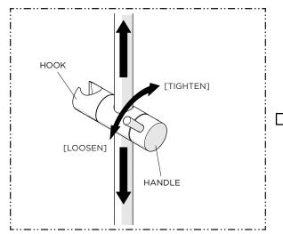
8. Loosen the HANDLE and adjust the HOOK on the BAR ASSEMBLY to the desired height then securely re-tighten the HANDLE.
