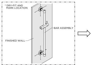
4. Dry-fit the BAR ASSEMBLY to the finished wall and mark the ideal location for installation; preferably over blocking or stud material.
