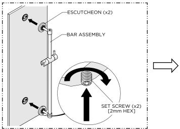
Slide the BAR ASSEMBLY onto the MOUNTING PLATES then thread and securely tighten the SET SCREWS on the ESCUTCHEONS.
