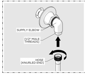
Thread and securely tighten the KNURLED end of the HOSE to the SUPPY ELBOW.
