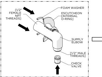
2. Slide the ESCUTCHEON and FOAM WASHER down the SUPPLY ELBOW.
