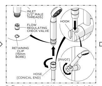
Thread and securely tighten the conical end of the HOSE to the HANDSHOWER then place it into the HOOK and pivot the HANDSHOWER to the desired position.
