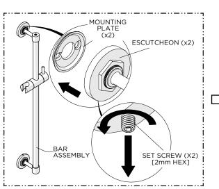
Loosen, but do NOT remove, the SET SCREW on each end of the BAR then remove the MOUNTING PLATES and ESCUTCHEONS.
