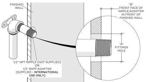
The front face of the NIPPLE/ADAPTER must be within 1/2" [13mm] and 7/8" [22mm] in order for the sliding ESCUTCHEON to properly fit onto the ELBOW.
