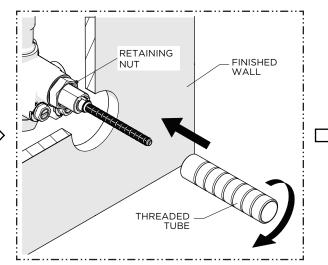
4. Thread the THREADED TUBE into the RETAINING NUT until snug.
