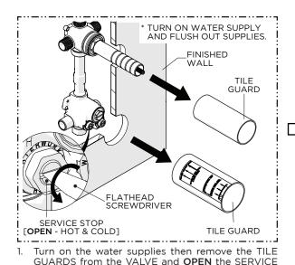
STOPS (hot & cold) and INTEGRATED DIVERTER
