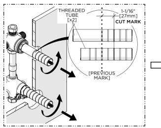
Remove the TUBES and cut them 1-1/16" [27mm] in front of the previous mark so the TUBES will protrude 1-1/16" [27mm] from the finished wall surface.
