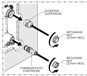
Unthread both RETAINING NUTS and remove both CARTRIDGES.
