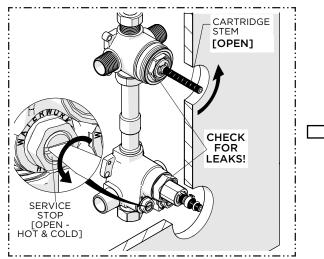
12. **OPEN** the SERVICE STOPS (hot & cold) and check for leaks. If no leaks are found, proceed and open the INTEGRATED DIVERTER VALVE
