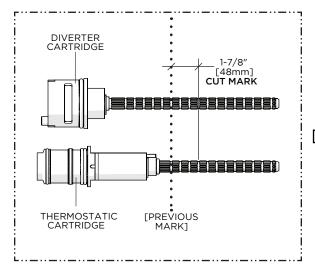
9. Carefully cut both CARTRIDGE STEMS 1-7/8" [48mm] in front of the previous mark so the STEMS will protrude 1-7/8" [48mm] from the finished wall surface.
