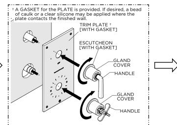
19. Firmly hold the TRIM PLATE against the finished wall then thread and securely tighten the GLAND COVERS onto the TUBES making sure to use the GASKETS provided.
