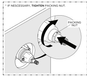
8. The PACKING NUT needs to be **securely** tightened to prevent a water leak from the CARTRIDGE STEM and create adequate rotational friction to maintain HANDLE position.
