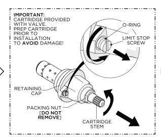
4. IMPORTANT: Leaving the PACKING NUT in place, unthread the LIMIT STOP SCREW until the O-RING is fully exposed then rotate the CARTRIDGE STEM counterclockwise to ensure the CARTRIDGE is drawn as close as possible to the RETAINING CAP.
