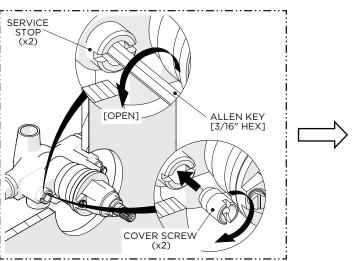
OPEN the SERVICE STOPS (hot & cold) then reinstall the COVER SCREWS (x2).
