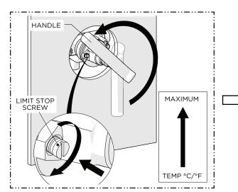
Open the VALVE to the maximum desired bathing temperature verified with a thermometer then turn the LIMIT STOP SCREW clockwise until it seats.
