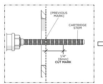
4. Carefully cut the CARTRIDGE STEM 1/4" [6mm] in front of the previous mark so the STEM will protrude 1/4" [6mm] from the finished wall surface.
