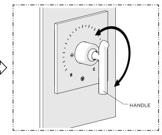
14. Operate the PRESSURE BALANCE TRIM and DIVERTER TRIM, if used, to ensure they are functioning properly.
