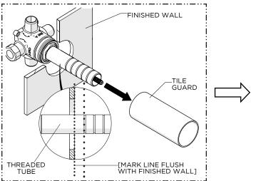
Remove the TILE GUARD when ready to install the TRIM then mark the THREADED TUBE where it protrudes past the finished wall.
