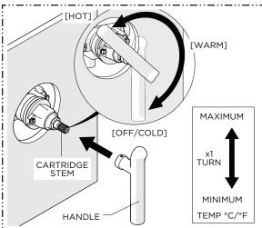
7. With the VALVE turned off, place the HANDLE on the CARTRIDGE STEM in the 6 o'clock position then turn the HANDLE counterclockwise through the cold, warm, and stopping at the hot position. Verify that a full range of temperatures exists.
