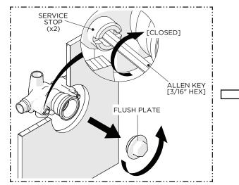
After the lines have been fully flushed, CLOSE the SERVICE STOPS (hot & cold) then unthread and remove the FLUSH PLATE.
