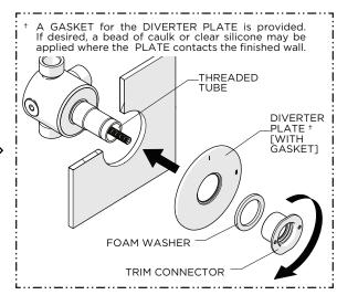
Firmly hold the DIVERTER PLATE against the finished wall then thread and securely tighten the TRIM CONNECTOR onto the THREADED TUBE making sure to use the FOAM WASHER provided.
