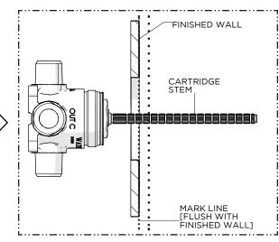
Mark the CARTRIDGE STEM where it protrudes past the finished wall.
