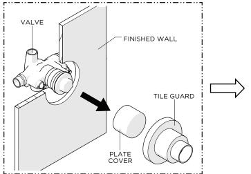
Remove the TILE GUARD and PLATE COVER from the VALVE when the TRIM is ready to be installed.
