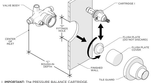
is packaged separately and provided with the VALVE. SET ASIDE UNTIL FINAL TRIM INSTALLATION!
