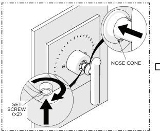
13. With the HANDLE fully seated, securely tighten the SET SCREWS (x2) then push the NOSE CONE into the GLAND COVER.
