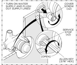
Turn on the water supplies then remove the COVER SCREWS (x2) and OPEN the SERVICE STOPS (hot & cold) to flush out the supply lines. CAUTION: FAILURE TO FLUSH THE SUPPLY LINES WILL PERMANENTLY DAMAGE THE CARTRIDGE AND VOID THE WARRANTY! REPEAT THE FLUSHING PROCESS AS NEEDED BEFORE FINAL TRIM INSTALLATION.
