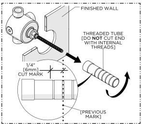
2. Remove the THREADED TUBE then cut it 1/4" [6mm] behind the previous mark so the TUBE will be 1/4" [6mm] below or recessed into the finished wall surface.
