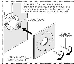
11. Slide the TRIM PLATE over the GLAND COVER then thread and securely tighten the SCREWS.
