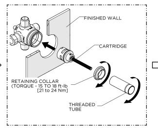
Thread the THREADED TUBE back onto the CARTRIDGE until snug.
