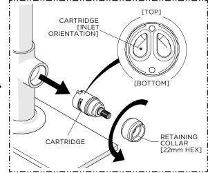
2. Unthread and remove the RETAINING COLLAR then pull the CARTRIDGE out.
