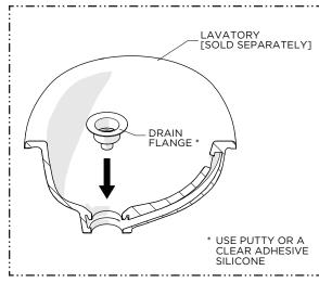
Set the DRAIN FLANGE into the LAVATORY (sold separately) using putty or a clear silicone.
