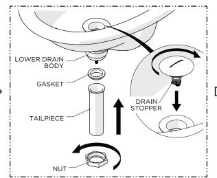
11. Re-install the DRAIN STOPPER and TAILPIECE using the GASKET and NUT provided.
