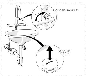
16. Close the HANDLE then open the DRAIN to drain the water.
