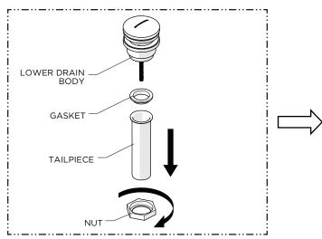
7. Unthread and remove the NUT, TAILPIECE, and GASKET from the LOWER DRAIN BODY.
