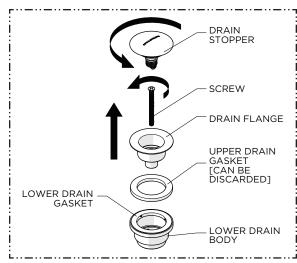
Remove the DRAIN STOPPER from the DRAIN FLANGE then unthread the SCREW from the LOWER DRAIN BODY.
