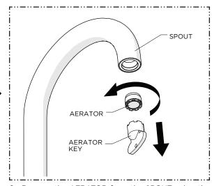
Remove the AERATOR from the SPOUT using the AERATOR KEY provided.
