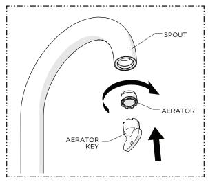
17. Re-install the AERATOR using the tool provided.
