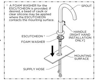
Insert the SUPPLY HOSES through the hole on the mounting surface making sure the FOAM WASHER provided is beneath the ESCUTCHEON.
