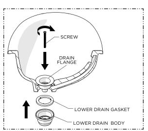
Insert the SCREW provided into the FLANGE then thread and securely tighten the SCREW into the LOWER DRAIN BODY making sure the LOWER DRAIN GASKET makes a full seal on the underside of the LAVATORY.
