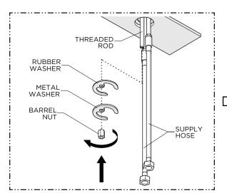
Slide the RUBBER and METAL WASHERS back onto the THREADED ROD then thread and securely tighten the BARREL NUT onto the ROD.
