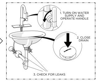
15. Turn on the water supply and operate the HANDLE to flush out the supply lines. Inspect all connections for leaks then close the DRAIN to ensure it functions properly.
