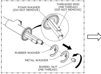
Remove the BARREL NUT, METAL WASHER, and RUBBER WASHER from the THREADED ROD.
