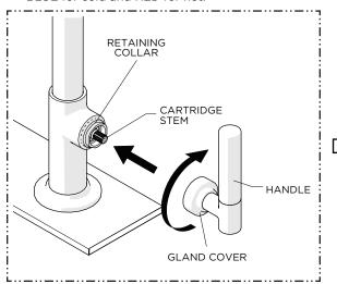
With the HANDLE held vertically, thread the GLAND COVER onto the RETAINING COLLAR until snug.
