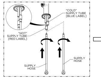
2. Thread and securely tighten the SUPPLY HOSES onto the SUPPLY TUBES on the SPOUT.
