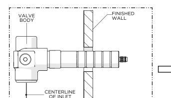
See the Installation Guidelines of the specific TRIM (sold separately) being used for the MAX and MIN rough-in depth dimensions.
