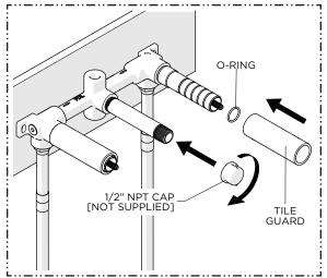
7. CAP the 1/2" NPT NIPPLE and attach the TILE GUARDS to the THREADED TUBES until construction is completed and the FAUCET is ready to be installed.
