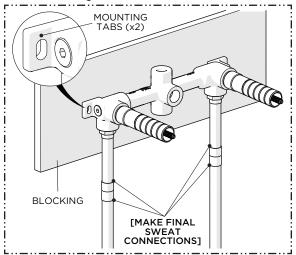
Verify the supplies are secure, level, and at the proper spread of 8" [203mm] prior to making final sweat connections. If necessary, utilize the MOUNTING TABS on the VALVE to secure it to blocking or other support material using appropriate SCREWS (not supplied).
