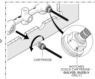
2. Unthread and remove the CARTRIDGE using a 21/32" [17mm] shower valve socket wrench.
