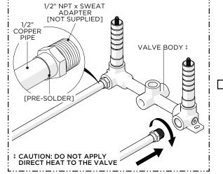
Pre-solder 1/2" COPPER PIPE to two 1/2" MALE NPT x SWEAT ADAPTERS (not supplied) then thread the ADAPTERS into the VALVE BODY.
