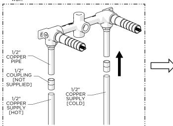
With the VALVE in the proper orientation, run 1/2" copper supply lines to the appropriate height and depth then connect to the VALVE using 1/2" COUPLINGS (not supplied).
