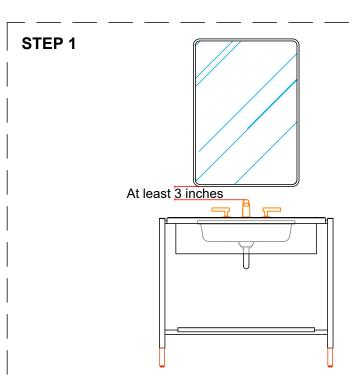
Choose your installation location to allow ample clearance to open the cabinet door. Allow at least 3 inches of clearance above or below the cabinet door for lighting and faucet clearance.
