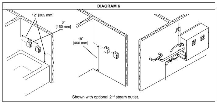
**5. INSTALL PRESSURE RELIEF SAFETY VALVE:** Install the pressure relief valve into its port on the generator. Install the safety valve within 6" [150] mm of the generator. Run a 3/4" copper line from the valve to a gravity flow drain. The pressure relief valve outlet must drain in accordance with local and national codes.
