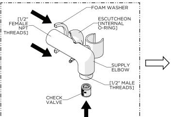
Slide the ESCUTCHEON and FOAM WASHER down the SUPPLY ELBOW.
