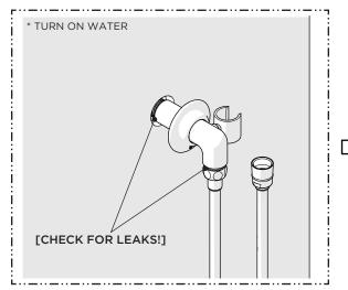
4. Turn on the water and a diverter/wall valve (sold separately) to flush out any debris in the supply line and inspect all connections for leaks then turn the water off.
