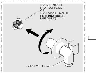
2. Thread and securely tighten the SUPPLY ELBOW onto the NIPPLE or BSPP ADAPTER.
