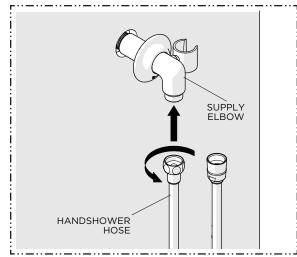
3. Thread and securely tighten the hex end of the HOSE to the ELBOW.
