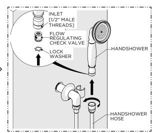
5. Thread and securely tighten the conical end of the HOSE to the HANDSHOWER then place it into the
