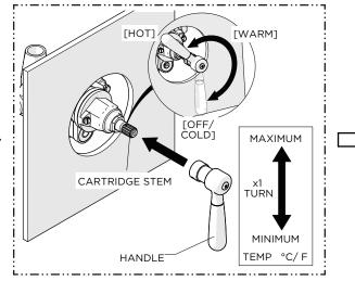
7. With the VALVE turned off, place the HANDLE on the CARTIRDGE STEM in the 6 o'clock position then turn the HANDLE counterclockwise through the cold, warm, and stopping at the hot position. Verify that a full range of temperatures exists.
