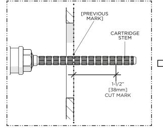
4. Carefully cut the CARTRIDGE STEM 1-1/2" [38mm] in front of the previous mark so the STEM will protrude 1-1/2" [38mm] from the finished wall surface.
