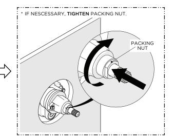
The PACKING NUT needs to be securely tightened to prevent a water leak from the CARTRIDGE STEM and create adequate rotational friction to maintain HANDLE position.
