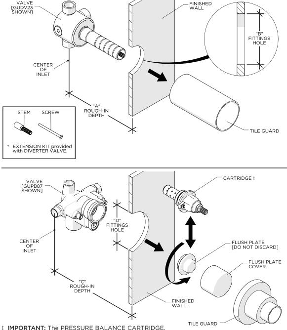
is packaged separately and provided with the VALVE. SET ASIDE UNTIL FINAL TRIM INSTALLATION!
