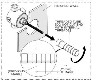
2. Remove the THREADED TUBE then cut it 1" [25mm] in front the previous mark so the STEM will protrude 1" [25mm] from the finished wall surface.
