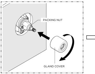
10. Thread and securely tighten the GLAND COVER onto the PACKING NUT.
