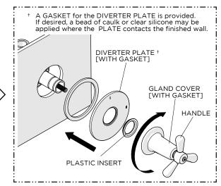
6. Firmly hold the DIVERTER PLATE against the finished wall then insert the PALASTIC INSERT into the PLATE and then with the HANDLE in the desired orientation, thread the GLAND COVER into the DIVERTER PLATE until it stops.
