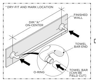
I. Ensure the TOWEL BAR is fully seated into the TOWEL BAR ENDS then dry-fit the assembly to the finished wall and mark the ideal location making sure to hold the BAR level.
