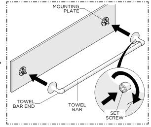
4. Slide the TOWEL BAR ENDS over the MOUNTING PLATES until they contact the finished wall then thread and securely tighten the SET SCREWS.
