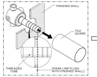
. Remove the TILE GUARD when ready to install the TRIM then mark the THREADED TUBE where it protrudes past the finished wall.
