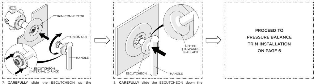
CAREFULLY slide the ESCUICHEON up the HANDLE to expose the UNION NUT then, with the HANDLE in the desired orientation, thread the NUT into the TRIM CONNECTOR until it stops. 8. **CAREFULLY** slide the ESCUTCHEON down the HANDLE to conceal the TRIM CONNECTOR.
