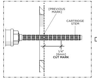
Carefully cut the CARTRIDGE STEM 1/4" [6mm] in front of the previous mark so the STEM will protrude 1/4" [6mm] from the finished wall surface.
