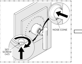
13. With the HANDLE fully seated, securely tighten the SET SCREWS (x2) then push the NOSE CONE into the GLAND COVER.
