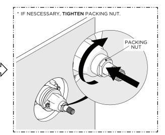
8. The PACKING NUT needs to be **securely** tightened to prevent a water leak from the CARTRIDGE STEM and create adequate rotational friction to maintain HANDLE position.
