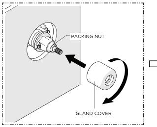
10. Thread and securely tighten the GLAND COVER onto the PACKING NUT.
