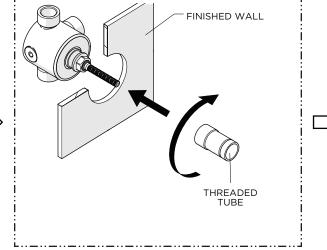
5. Thread the THREADED TUBE back onto the CARTRIDGE until it stops.
