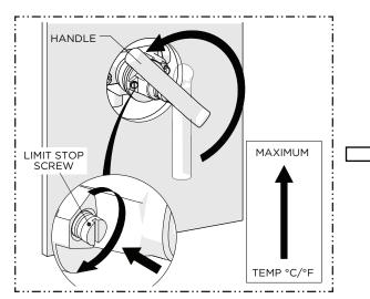
9. Open the VALVE to the **maximum** desired bathing temperature verified with a thermometer then turn the LIMIT STOP SCREW clockwise until it seats.
