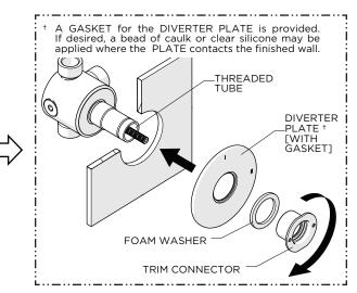
Firmly hold the DIVERTER PLATE against the finished wall then thread and securely tighten the TRIM CONNECTOR onto the THREADED TUBE making sure to use the FOAM WASHER provided.
