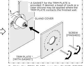
11. Slide the TRIM PLATE over the GLAND COVER then thread and securely tighten the SCREWS.
