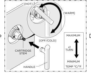
7. With the VALVE turned off, place the HANDLE on the CARTIRDGE STEM in the 6 o'clock position then turn the HANDLE counterclockwise through the cold, warm, and stopping at the hot position. Verify that a full range of temperatures exists.
