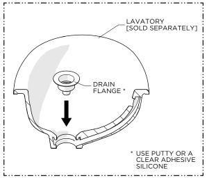
11. Set the DRAIN FLANGE into the lavatory (sold separately) using putty or a clear silicone.
