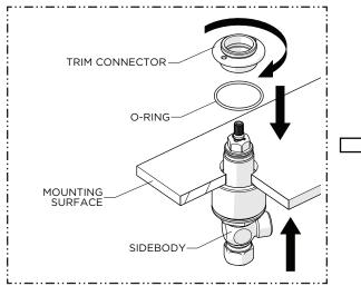
5. Using the O-RING provided, thread the TRIM CONNECTOR back onto the SIDEBODY until it stops then let it rest on the mounting surface.
