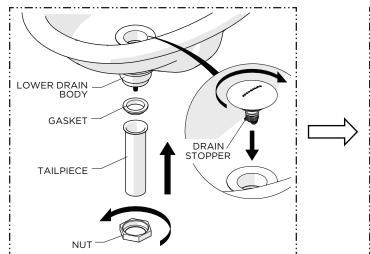
13. Re-install the DRAIN STOPPER and TAILPIECE using the GASKET and NUT provided.
