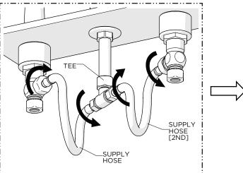
8. Connect the SIDEBODIES to the TEE using the SUPPLY HOSES provided. Securely tighten the HOSES and ensure they are not pinched/kinked.
