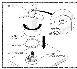
Using the GASKET provided, place the HANDLE over the CARTRIDGE STEM then thread and securely tighten the GLAND COVER onto the TRIM CONNECTOR.
