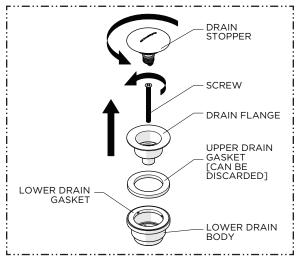
Remove the DRAIN STOPPER from the DRAIN FLANGE then unthread the SCREW from the LOWER DRAIN BODY.
