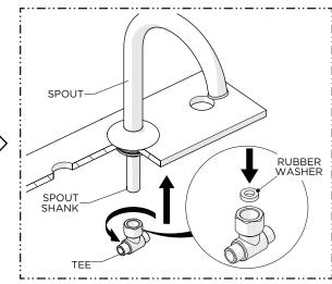
Thread and securely tighten the TEE onto the SHANK making sure to use the RUBBER WASHER provided.
