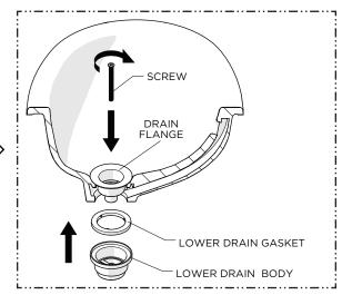
12. Insert the SCREW provided into the FLANGE then thread and securely tighten the SCREW into the LOWER DRAIN BODY making sure the LOWER DRAIN GASKET makes a full seal on the underside of the LAVATORY.
