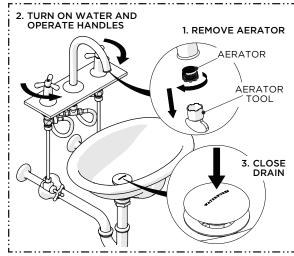
15. Remove the AERATOR, turn on the water to flush out the supply lines, inspect all connections for leaks and close the DRAIN to ensure it functions properly.
