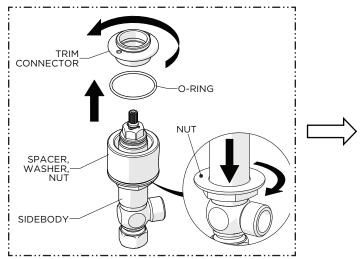
Unthread and remove the TRIM CONNECTOR with the O-RING beneath it then fully thread the NUT down the SIDEBODY.
