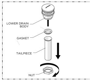
Unthread and remove the NUT, TAILPIECE, and GASKET from the LOWER DRAIN BODY.
