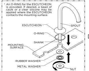
Insert the SHANK through the hole on the mounting surface making sure the O-RING provided is beneath the ESCUTCHEON then reattach the RUBBER and METAL WASHERS and securely tighten the NUT.
