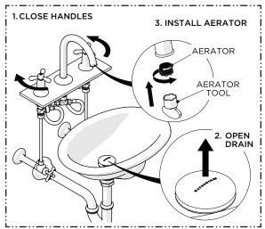
16. Close the HANDLES, open the DRAIN, and reinstall the AERATOR.
