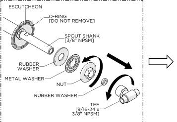
Remove the TEE, NUT, METAL WASHER, and RUBBER WASHER from the SPOUT SHANK.
