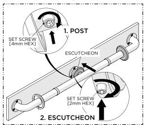
10. Securely tighten the SET SCREW on the center POST then slide the ESCUTCHEON down to conceal the MOUNTING PLATE and securely tighten the SET SCREW on the ESCUTCHEON.
