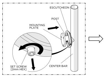
Loosen, but do NOT remove, the SET SCREW on the ESCUTCHEON of the CENTER BAR then slide the ESCUTCHEON up the POST to expose the MOUNTING PLATE.
