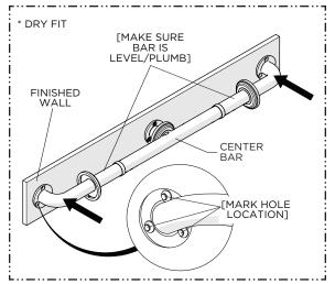
7. Dry-fit the GRAB BAR to the finished wall, making sure it is level, plumb, or at the desired orientation. and mark the hole locations.
