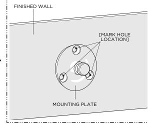
3. Place the MOUNTING PLATE on the finished wall at the desired position and mark the hole locations.
