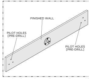
8. Using the previous marks as a reference, drill pilot holes into the blocking or stud material to accommodate the SCREWS provided.
