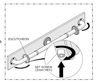
11. Slide the ESCUTCHEONS on the GRAB BAR ENDS down to conceal the MOUNTING PLATES then securely tighten the SET SCREWS.
