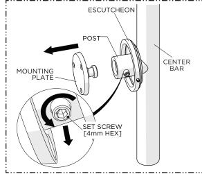
2. Loosen, but do NOT remove, the SET SCREW at the base of the POST then remove the MOUNTING PLATE.
