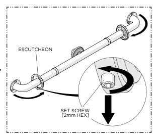
6. Loosen, but do NOT remove, the SET SCREWS on the ESCUTCHEONS of the GRAB BAR ENDS then slide the ESCUTCHEONS up the ENDS to expose the MOUNTING PLATES.
