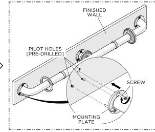
9. Secure the GRAB BAR to the wall using the SCREWS provided.
