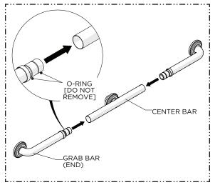
Assemble the GRAB BAR ENDS to the CENTER BAR making sure the ENDS are fully seated and properly aligned.
