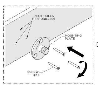
4. Using the previous marks as a reference, drill pilot holes into the blocking or stud material to accommodate the SCREWS provided then install the MOUNTING PLATE.
