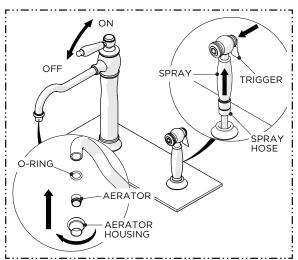
11. Re-install the AERATOR then operate the SPOUT and SPRAY to ensure they operate and function properly.
