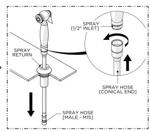
6. Thread and securely tighten the SPRAY HOSE onto the SPRAYER then, from the top, insert the HOSE into the SPRAY RETURN making sure the SPRAY can rest properly.
