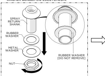
4. SPRAY RETURN: Unthread and remove the NUT. METAL WASHER, and RUBBER WASHER from the SPRAY RETURN SHANK.
