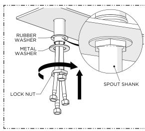
3. Slide the RUBBER WASHER, METAL WASHER, and LOCK NUT over the HOSES and SPOUT SHANK then thread and securely tighten the LOCK NUT onto the SHANK.
