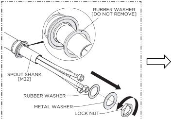
SPOUT: Unthread and remove the LOCK NUT from the SPOUT SHANK then remove the METAL WASHER and RUBBER WASHER.
