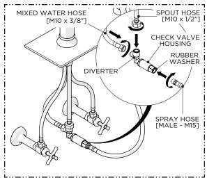
Thread the MIXED WATER and SPOUT HOSES to the DIVERTER TEE, then thread and securely tighten the SPRAY HOSE into the CHECK VALVE HOUSING.
