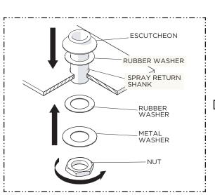
Insert the SPRAY RETURN SHANK through the hole on the MOUNTING SURFACE making sure the RUBBER WASHER provided is beneath the ESCUTCHEON, then re-install the RUBBER WASHER, METAL WASHER and securely tighten the NUT.
