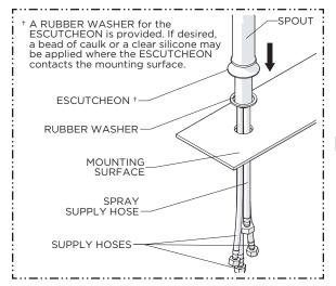
Insert the HOSES and SPOUT SHANK through the hole on the mounting surface making sure the RUBBER WASHER provided is beneath the ESCUTCHEON.
