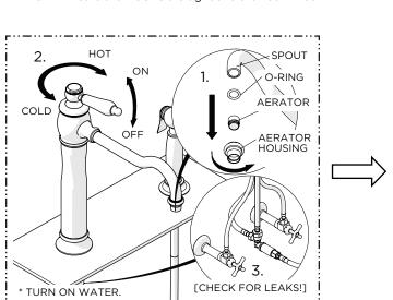
10. Remove the AERATOR then turn on the water supply to flush out any debris in the supply lines and inspect all connections for leaks.
