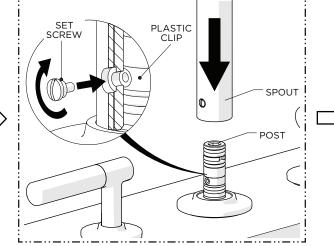
2. When replacing the SPOUT, the SET SCREW must properly align with the hole on the PLASTIC CLIP to securely hold the SPOUT in position.
