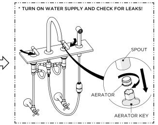
15. Unthread and remove the AERATOR then turn on the water supply and open the FAUCET to flush out any debris in the supply lines prior to operating the SPRAYER. Inspect all connections for leaks.
