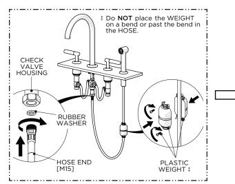
13. Using the RUBBER WASHER provided, thread the SPRAY HOSE into the CHECK VALVE HOUSING then attach the WEIGHT to a **straight** section of the HOSE that is opposite the HOUSING/TEE and verify the SPRAYER sits properly in the HOLDER.
