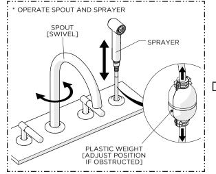
17. Pull out the SPRAYER and rotate the SPOUT to ensure they function properly and the WEIGHT can move freely beneath the cabinet.
