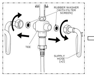
16. Turn off the FAUCET and unthread both the SUPPLY HOSES from the TEE to remove and clean the WASHER WITH FILTER SCREENS then reinstall the WASHERS and HOSES.
