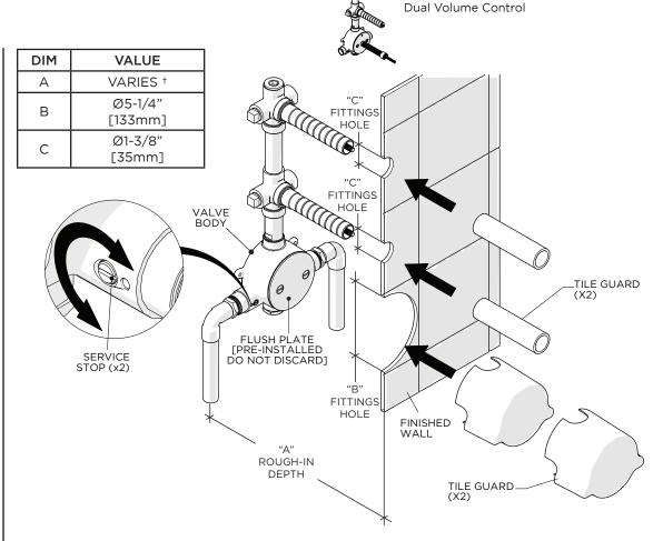
Refer to the Installation Guidelines of the specific TRIM being used for the MAXIMUM and MINIMUM rough-in depth dimensions.
