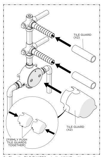
Place the TILE GUARDS onto the VALVE making sure they are FULLY seated and do NOT remove until construction is completed. Ensure the TILE GUARDS for the THERMOSTATIC VALVE are firmly push together before attaching them to the VALVE.
