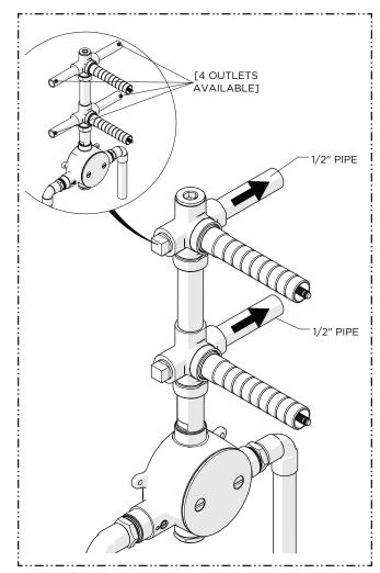
4. Run 1/2" copper lines from the side outlets being used to the desired end fittings (sold separately) making sure to secure all piping and fittings.
