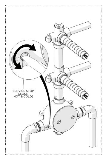
7. After the supply lines have been fully flushed, turn off the water and close the SERVICE STOPS (hot & cold).
