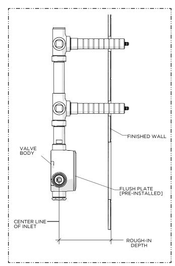
See the Installation Guidelines of the specific TRIM (sold separately) being used for the MAX and MIN rough-in depth dimensions.
