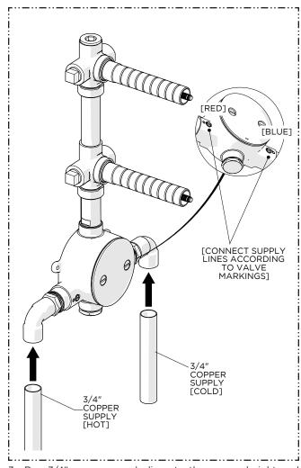
Run 3/4" copper supply lines to the proper height and depth of the VALVE INLETS making sure they are piped according to the VALVE markings and all piping and fittings are properly secured.
