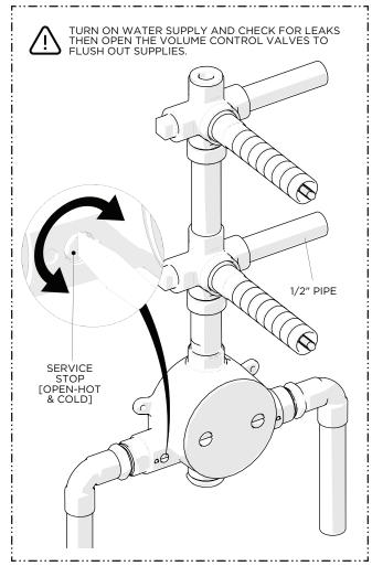
Turn on the water supplies then open the SERVICE STOPS (hot & cold) and open the VOLUME CONTROL VALVES to flush out the lines and check for leaks.
