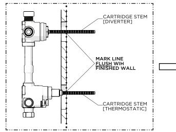
7. Mark both CARTRIDGE STEMS where they protrude past the finished wall.
