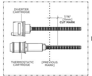
9. Carefully cut both CARTRDGE STEMS 7/16" [11mm] in front of the previous mark so the STEMS will protrude 7/16" [11mm] from the finished wall surface.
