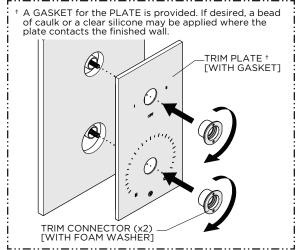
19. Firmly hold the TRIM PLATE against the finished wall then thread and securely tighten the TRIM CONNECTORS onto the TUBES making sure to use the FOAM WASHERS provided.
