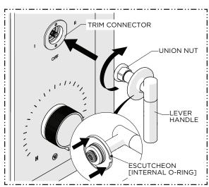
22. CAREFULLY slide the ESCUTCHEON up the LEVER HANDLE to expose the UNION NUT then thread the NUT into the TRIM CONNECTOR until it stops.
