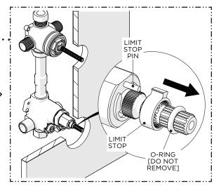
IF THE MAXIMUM BATHING TEMPERATURE IS NOT CORRECT OR NEEDS TO BE ADJUSTED:
