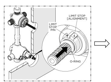
15. Slide the LIMIT STOP and O-RING back down the STEM making sure to properly align the LIMIT STOP with the LIMIT STOP PIN.
