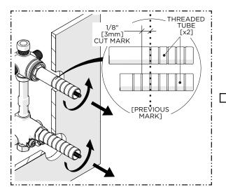
6. Remove the TUBES and cut them 1/8" [3mm] behind the previous mark so the TUBES will be 1/8" [3mm] below or recessed into the finished wall surface.
