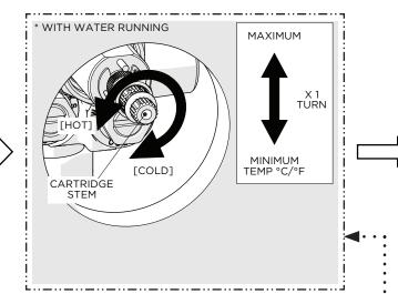
13. With water running, slowly rotate the THERMOSTATIC CARTRIDGE STEM clockwise to attain full cold then rotate it counterclockwise to attain full hot. Verify that a full range of temperatures exists.
