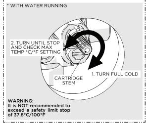
16. Re-open the DIVERTER VALVE then turn the THERMOSTATIC CARTRIDGE STEM clockwise to full cold then counterclockwise until it stops. Verify the maximum desired bathing temperature set in the previous step then turn the water off.
