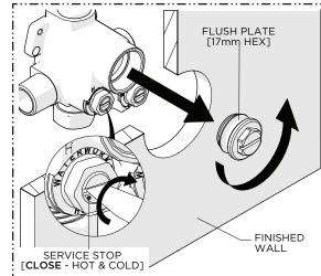
2. After the lines have been fully flushed, CLOSE the SERVICE STOPS (hot & cold) then unthread and remove the FLUSH PLATE.
