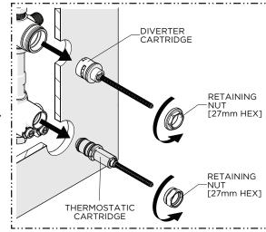
8. Unthread both RETAINING NUTS and remove both CARTRIDGES.
