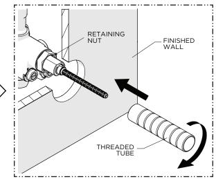
4. Thread the THREADED TUBE into the RETAINING NUT until it stops.
