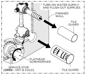
CAUTION: FAILURE TO FLUSH THE SUPPLY LINES WILL PERMANENTLY DAMAGE THE CARTRIDGE AND VOID THE WARRANTY! REPEAT THE FLUSHING PROCESS AS NEEDED BEFORE FINAL TRIM INSTALLATION.
