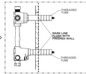
5. Mark both TUBES where they protrude past the finished wall.
