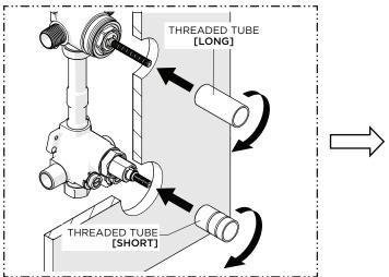
18. Thread the THREADED TUBES back into the RETAINING NUTS until they stop.
