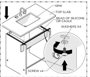
8. Add a bead of caulk or clear silicone on the top surface of the BASE. Place the TOP SLAB over the BASE with the SINK positioned inside the FRAME and bump against the wall. From underneath the slab, fasten the TOP SLAB to the FRAME with the SCREWS and WASHERS provided.
