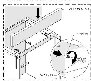
Carefully install the APRON SLAB into the notches on each LEG, using the screws and washers provided, fasten the FRAME to the APRON SLAB.
