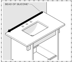
9. If desired, a bead of caulk or a clear silicone may be applied where the TOP SLAB contacts the finished
