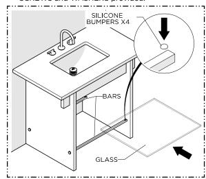
11. Place one SILICONE BUMPER on top of each BAR side 1" away from the LEG's inner surface, Install the GLASS on top of the BARS to finish the setup.
