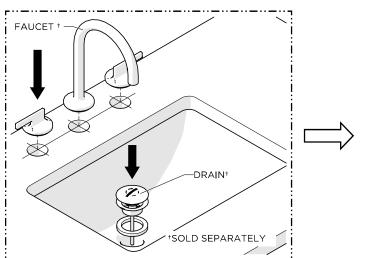
7. Install the FAUCET and the DRAIN on the TOP SLAB with SINK.
