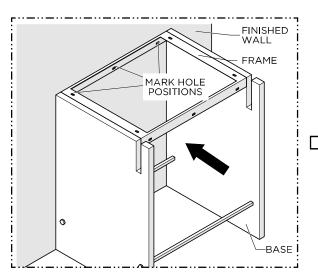
4. Dry fit the BASE to the desired position against the wall ensuring the LEGS are level and mark the FRAME's hole locations. Remove the BASE. Drill pilot holes in the wall in the marked locations. Install plastic WALL ANCHORS [not supplied] if no stud or blocking is present.
