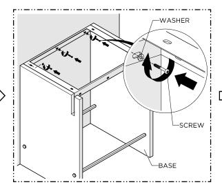
Move BASE back into position and fasten the FRAME with the SCREWS and WASHERS provided.
