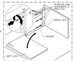
2. Fasten the FRAME to the pre-installed marble anchors of the LEFT LEG and RIGHT LEG using the WASHERS & SCREWS supplied.
