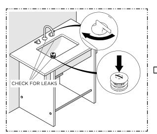
10. Make final FAUCET and DRAIN connections (if applicable). Turn on the water and operate the drain and faucet fittings to ensure proper operation. Check all connections for leaks.
