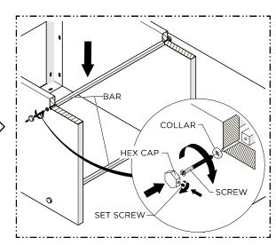
Use one SCREW and COLLAR to fasten the BAR to one LEG. Cover the COLLAR with the HEX CAP and secure it with the SET SCREW. Repeat on the other LEG. Install the second BAR following the same process. This completes the washstand BASE.
