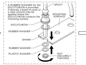
2. Insert the SHANK through the hole on the mounting surface making sure the RUBBER WASHER provided is beneath the ESCUTCHEON then re-install the LOWER DECK WASHERS and securely tighten the NUT.
