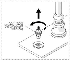
3. Unthread and remove the CARTRIDGE using a 21/32" [17mm] shower valve socket wrench.
