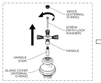
4. Remove the INDICE then unthread the SCREW and remove the HANDLE and HANDLE STEM.
