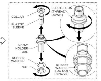
12. Remove the COLLAR, PLASTIC SLEEVE, NUT and RUBBER WASHER from the SPRAY HOLDER TUBE then partially unthread, but do **NOT** remove, the ESCUTCHEON or the RUBBER WASHER beneath.
