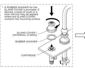
8. Using the RUBBER WASHER provided, thread the GLAND COVER back onto the CARTRIDGE until it contacts the mounting surface.
