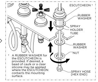
14. Insert the HOSE and the SPRAY HOLDER TUBE though the hole on the mounting surface making sure the RUBBER WASHER is beneath the ESCUTCHEON then re-install the RUBBER WASHER and securely tighten the NUT.
