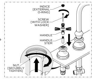
9. Fully insert the HANDLE STEM into the GLAND COVER and place the HANDLE onto the STEM then thread and securely tighten the SCREW. Ensure the HANDLE is in the desired orientation then securely tighten the NUT and install the INDICE.
