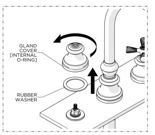
2. Unthread and remove the GLAND COVER and RUBBER WASHER.
