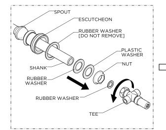
I. Unthread and remove the TEE, NUT, and LOWER DECK WASHERS from the SPOUT SHANK. NOTE: Do NOT remove the RUBBER WASHER beneath the ESCUTCHEON or discard the RUBBER WASHER provided with the TEE.
