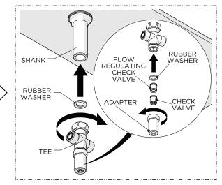
3. Using the RUBBER WASHER provided, thread and securely tighten the TEE back onto the SHANK.
