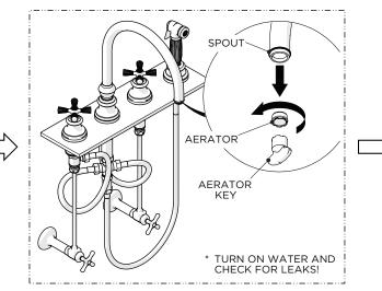
17. Unthread and remove the AERATOR then turn on the water to flush out any debris in the supply lines and inspect all connections for leaks.
