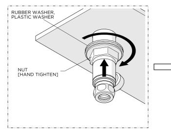
Hand-tighten the NUT against the underside of the mounting surface.
