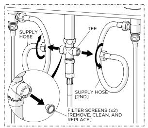
Turn off the water and unthread both the SUPPLY HOSES from the TEE to remove and clean the FILTER SCREENS then re-install the SCREENS and HOSES.
