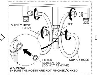
11. Connect the SIDEBODIES to the TEE using the SUPPLY HOSES provided. Securely tighten the HOSES and ensure they are not pinched/kinked.
