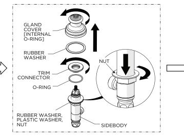
5. Unthread and remove the GLAND COVER, RUBBER WASHER, TRIM CONNECTOR and O-RING from the SIDEBODY then fully thread the NUT down.
