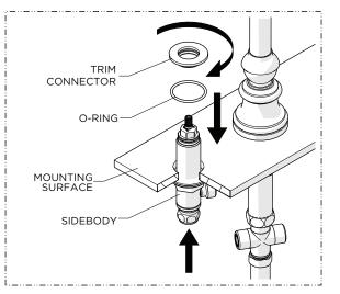
6. Using the O-RING provided, thread the TRIM CONNECTOR back onto the SIDEBODY until it stops then let it rest on the mounting surface.
