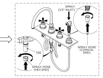
15. Thread and securely tighten the SPRAY HOSE [conical end] onto the SPRAY and insert the HOSE into the SPRAY HOLDER until it stops then thread and securely tighten the HOSE [hex end] onto the TEE.
