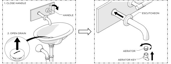
24. Close the HANDLE then open the DRAIN to drain the water.
