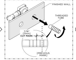
2. Remove the THREADED TUBE then cut it 7/16" [11mm] behind the previous mark.
