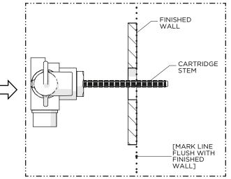
Mark the CARTRIDGE STEM where it protrudes 3 past the finished wall.
