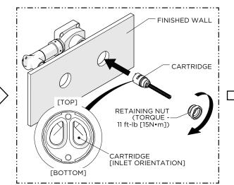
Insert the CARTRIDGE back into the VALVE in 5. the proper orientation then thread and securely tighten the RETAINING NUT.
