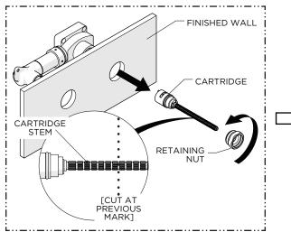
4. Remove the RETAINING NUT and CARTRIDGE then cut the CARTRIDGE STEM at the previous mark.
