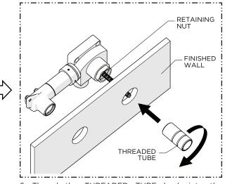
6. Thread the THREADED TUBE back into the RETAINING NUT until it stops.
