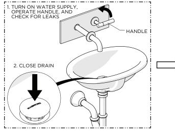
23. Turn on the water supply and operate the HANDLE to flush out the supply lines, and inspect all connections for leaks then close the DRAIN to ensure it functions properly.
