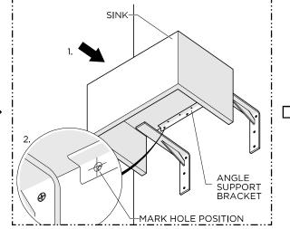
2. Dry fit the SINK with ANGLE SUPPORT BRACKET ensuring it is level and re-adjust or shim (not included) if necessary. Mark the three holes locations for the ANGLE SUPPORT BRACKET. Remove the SINK and drill pilot holes for #12 WOOD SCREWS.
