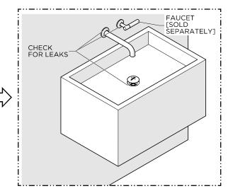
Turn on the water and operate the drain and faucet [sold separately] to ensure proper operation. Check all connections for leaks. If desired, a bead of caulk or clear silicone may be applied where the SINK contacts the finished wall.
