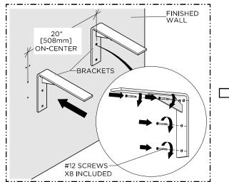
1. Dry fit the BRACKETS to the FINISHED WALL and mark the location of the mounting holes. Make sure to hold the BRACKETS level. Drill pilot holes for the #12 WOOD SCREWS provided. Secure the BRACKETS using the #12 WOOD SCREWS.
