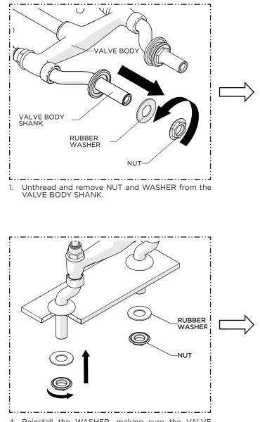
4. Reinstall the WASHER, making sure the VALVE BODY is in proper orientation then securely tighten the NUT onto the VALVE BODY.
