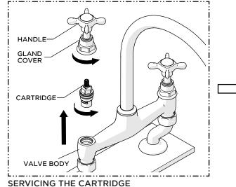
1. Unthread the GLAND COVER and pull the HANDLE off to expose the CARTRIDGE then unthread and remove the CARTRIDGE using a 21/32" [17mm] wrench.
