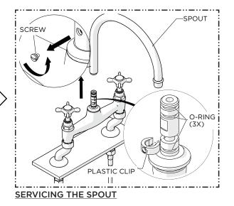
2. Remove the SCREW at the base of the SPOUT then remove the SPOUT to expose the POST and external O-RINGS.
