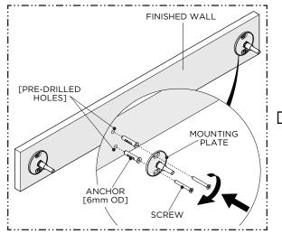
Using the previous marks as a reference, install the MOUNTING PLATES using the ANCHORS, if necessary, and SCREWS provided.
