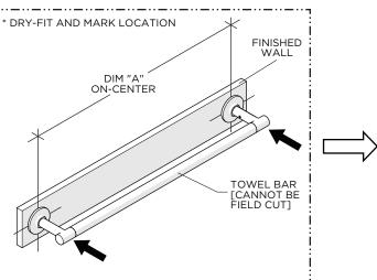
Dry-fit the TOWEL BAR to the finished wall and mark the ideal location making sure to hold the BAR level.
