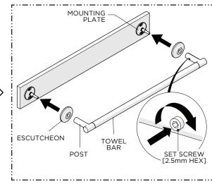
Slide the ESCUTCHEONS and POSTS onto the MOUNTING PLATES then thread and securely tighten the SET SCREWS.
