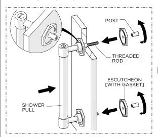
Slide the ESCUTCHEONS onto the THREADED RODS then thread and securely tighten the POSTS.
