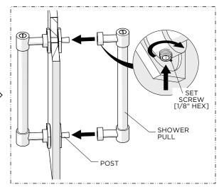
Slide the PULL onto the POSTS until it contacts the ESCUTCHEONS then thread and securely tighten the SET SCREWS.
