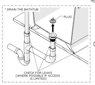
14. Drain the BATHTUB and inspecting all connections above and below the finished floor for leaks where possible if access is limited.
