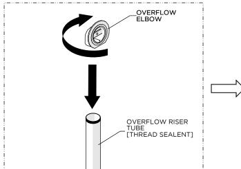
8. Apply thread sealant or pipe dope to the threads on the RISER TUBE then thread and securely tighten the ELBOW onto the TUBE.
