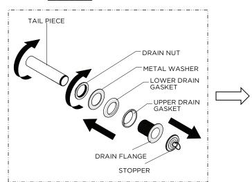
Remove the STOPPER, UPPER and LOWER DRAIN GASKETS, WASHERS, NUT and TAILPIECE from the DRAIN FLANGE.
