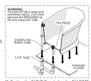
12. Position the BATHTUB and align the TAILPIECE and OVERFLOW RISER TUBE with the DRAIN HUBS then carefully lower the BATHTUB until it rests on the finished floor.
