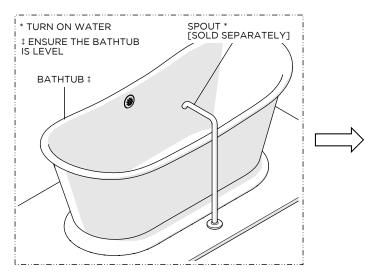
13. Verify the BATHTUB is level and, if needed, add shims then fill the BATHTUB until water enters the overflow hole.
