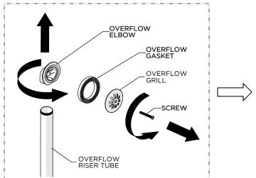
7. Unthread and remove the SCREW, OVERFLOW GRILL, and OVERFLOW GASKET, Remove OVERFLOW RISER PIPE from OVERFLOW FLBOW.
