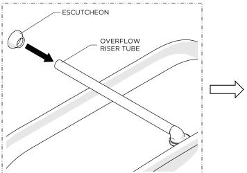
10. Slide the ESCUTCHEON onto the OVERFLOW RISER TUBE.
