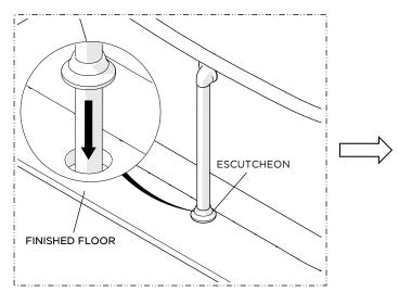
16. Slide the ESCUTCHEON down the OVERFLOW RISER TUBE until it contacts the finished floor.
