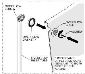
9. Apply a generous bead of silicone sealant to both sides of the OVERFLOW GASKET then assemble the OVERFLOW RISER TUBE to the BATHTUB and securely tightening the SCREW.
