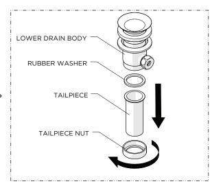
Unthread and remove the NUT, TAILPIECE, and the RUBBER WASHER from the LOWER DRAIN BODY.
