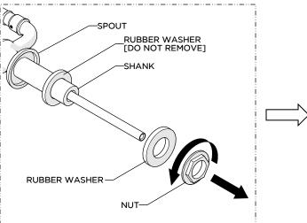
Unthread and remove the NUT and lower deck WASHER from the SHANK.
