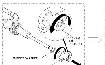
Loosen, but do NOT remove the PACKING NUT at the base of the TEE then remove the TEE and RUBBER WASHER from the SHANK.
