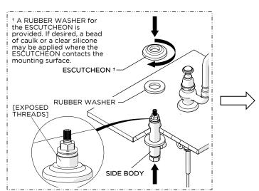
Using the RUBBER WASHER provided, thread the ESCUTCHEON back onto the SIDEBODY and let it rest on the mounting surface.
