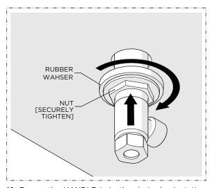
12. Ensure the HANDLE is in the desired orientation then thread and securely tighten the NUT against the underside of the mounting surface.
