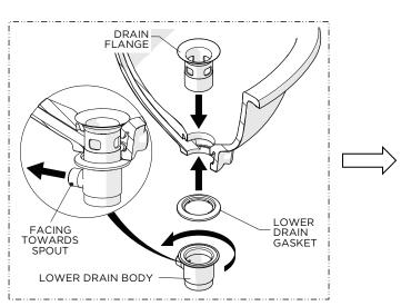
17. Set the DRAIN FLANGE into the lavatory (sold separately) using putty or a clear silicone and attach the LOWER DRAIN GASKET then securely tighten the LOWER DRAIN BODY onto the FLANGE.
