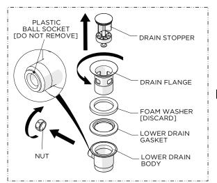
Unthread and remove the DRAIN STOPPER, DRAIN FLANGE, LOWER DRAIN GASKET, and NUT from the LOWER DRAIN BODY.
