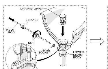
19. Making sure the BALL SOCKET is in place, insert the PIVOT ROD into the DRAIN BODY and securely tighten the NUT then insert the STOPPER into the FLANGE making sure the SCREW rests on top of the PIVOT ROD. Adjust the SCREW if needed.
