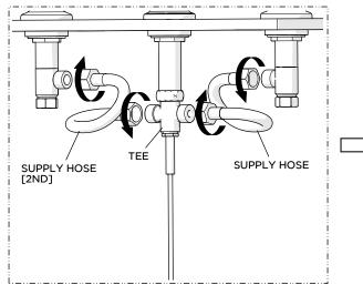
14. Connect the SIDEBODIES to the TEE using the SUPPLY HOSES and RUBBER WASHER provided. Securely tighten the HOSES and ensure they are not pinched/kinked.
