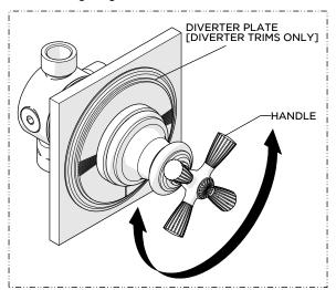
10. Turn on the water supply and operate the HANDLE to ensure that it is functioning properly.
