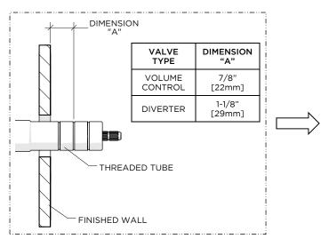
Remove the TILE GUARD when ready to install the TRIM then mark the THREADED TUBE in front of the finished wall at the correct length listed for the VALVE being used.
