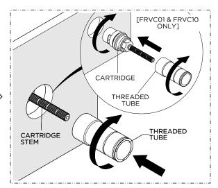
Thread and securely tighten the THREADED TUBE back onto the VALVE.
