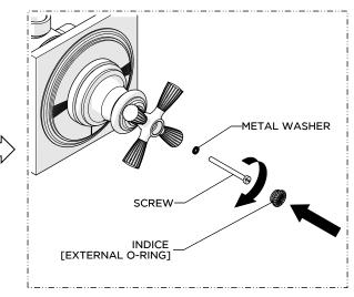
Thread and securely tighten the SCREW with the METAL WASHER provided then insert the INDICE onto the HANDLE.
