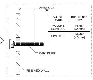
Mark the CARTRIDGE STEM in front of the finished wall at the correct length listed for the VALVE being used.
