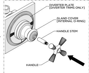
Insert the HANDLE STEM into the GLAND COVER, place the HANDLE onto the STEM in the desired orientation.
