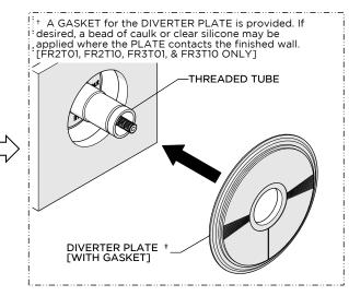
FR2T01, FR2T10, FR3T01 AND FR3T10 ONLY: Slide the DIVERTER PLATE over the THREADED TUBE and hold it against the finished wall.
