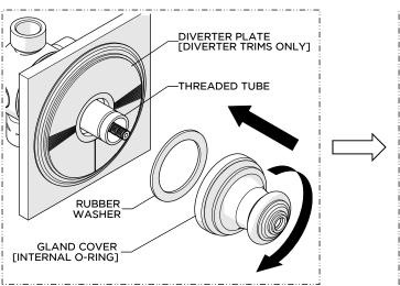
7. Making sure the RUBBER WASHER is beneath the GLAND COVER, thread and securely tighten the GLAND COVER onto the THREADED TUBE.
