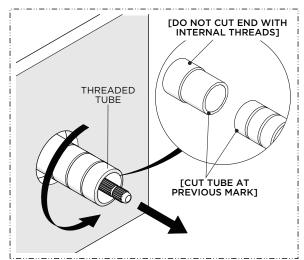
2. Remove the THREADED TUBE then cut the TUBE at the previous mark.
