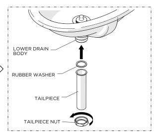
Re-install the TAILPIECE using the WASHER and NUT provided.
