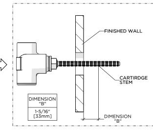
3. Mark the CARTRIDGE STEM in front of the finished wall at the length listed.
