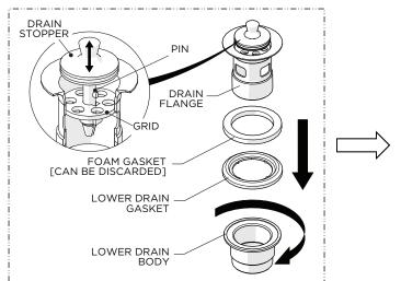
Unthread and remove the LOWER DRAIN BODY and LOWER DRAIN GASKET from the DRAIN FLANGE.
