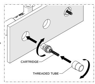
6. Repeat Steps 1 - 5 to cut the second (2ND) THREADED TUBE and CARTRIDGE STEM.
