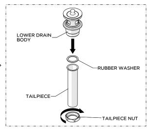
12. Unthread and remove the NUT, TAILPIECE, and the RUBBER WASHER from the LOWER DRAIN BODY.
