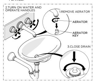
17. Removed the AERATOR, turn on the water to flush out the supply lines, and inspect all connections for leaks. Close the DRAIN to ensure it functions properly then turn off the water and re-install the AERATOR.
