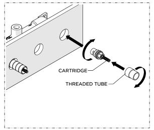
5. Thread and securely tighten the CARTRIDGE back into the VALVE then thread the THREADED TUBE back onto the CARTRIDGE.
