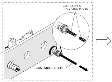
4. Remove the CARTRIDGE using a 21/32" [17mm] shower valve socket wrench (not provided) then cut the STEM at the previous mark.
