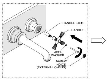
10. Fully insert the STEM into the GLAND COVER and place the HANDLE in the desired orientation onto the STEM then thread and securely tighten the SCREW and install the INDICE.
