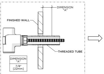
1. Remove the TILE GUARD when ready to install the TRIM then mark the THREADED TUBE in front of the finished wall at the length listed.
