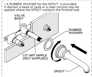
8. Using the RUBBER WASHER provided, thread and securely tighten the SPOUT onto the NIPPLE (not supplied).
