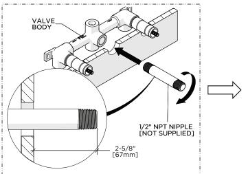
7. Thread a 1/2" NPT x 1/2" NPT NIPPLE (not supplied) of appropriate length into the VALVE and ensure the front face of the NIPPLE projects 2-5/8" [67mm] from the surface of the finished wall.
