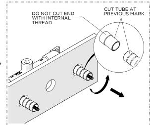
2. Remove the THREADED TUBE then cut the TUBE at the previous mark.
