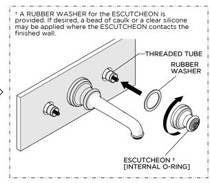
Using the RUBBER WASHER provided, thread and securely tighten the ESCUTCHEON onto the THREADED TUBE.
