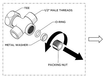
4. Remove the PACKING NUT, METAL WSAHER and O-RING from the TEE to prevent the GUIDE TUBE in the SPOUT from damaging the O-RING.
