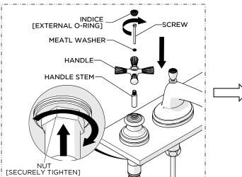
14. Fully insert the HANDLE STEM into the GLAND COVER and place the HANDLE onto the STEM then thread and securely tighten the SCREW. Ensure the HANDLE is in the desired orientation then securely tighten the NUT and install the INDICE.
