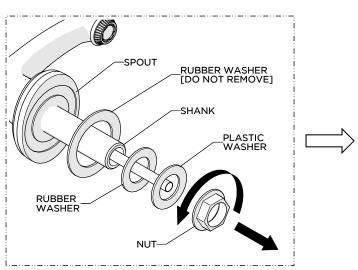
Unthread and remove the NUT and lower deck WASHERS from the SHANK.
