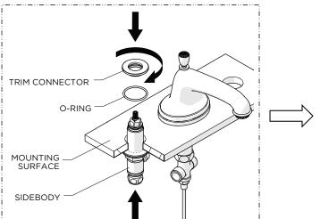
11. Using the O-RING provided, thread the TRIM CONNECTOR back onto the SIDEBODY then let it rest on the mounting surface.
