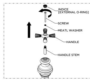
9. Remove the INDICE then unthread and remove the SCREW, METAL WASHER, HANDLE and STEM.
