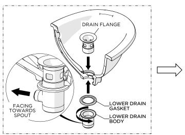
19. Set the DRAIN FLANGE into the lavatory (sold separately) using putty or a clear silicone and attach the LOWER DRAIN GASKET then securely tighten the LOWER DRAIN BODY onto the FLANGE.
