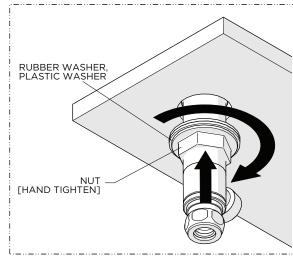
12. Hand-tighten the NUT against the underside of the mounting surface.
