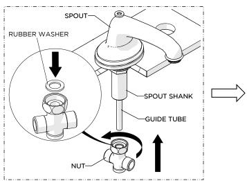
Thread and securely tighten the TEE onto the SHANK making sure to use the RUBBER WASHER provided.
