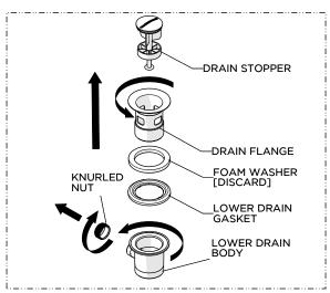
18. Unthread and remove the LOWER DRAIN BODY, LOWER DRAIN GASKET, and the DRAIN STOPPER from the DRAIN FLANGE. Unthread and remove the KNURLED NUT from the LOWER DRAIN BODY.
