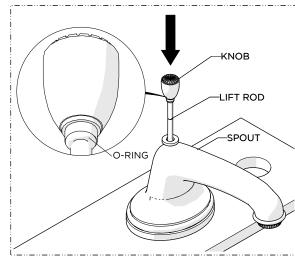
Insert the LIFT ROD into the top of the SPOUT making sure the O-RING is beneath the KNOB.
