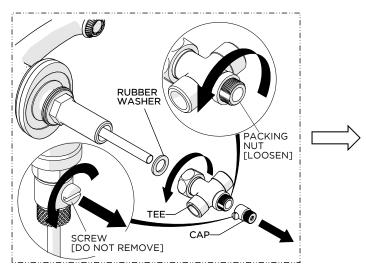
Loosen but do NOT remove the SCREW on the CAP then remove the CAP. Loosen but do NOT remove the PACKING NUT at the base of the TEE then remove the TEE and RUBBER WASHER from the SHANK.
