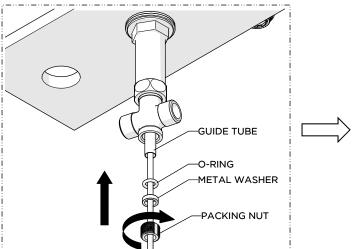
7. Insert the O-RING and METAL WASHER into the PACKING NUT.
