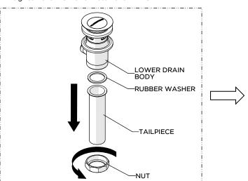
17. Unthread and remove the NUT, TAILPIECE, and the RUBBER WASHER from the LOWER DRAIN BODY.
