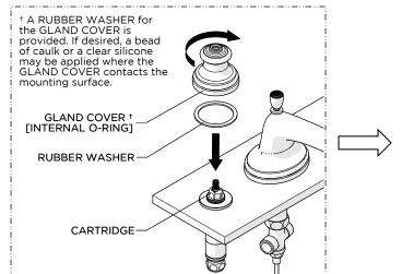
13. Using the RUBBER WASHER provided, thread the GLAND COVER back onto the CARTRIDGE until it contacts the mounting surface.
