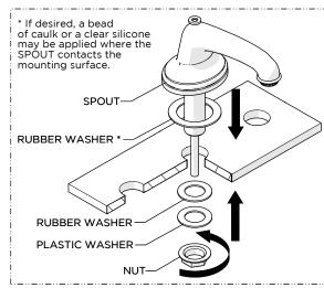
Insert the SHANK through the hole on the mounting surface making sure the RUBBER WASHER is beneath the SPOUT then reattach the WASHERS and securely tighten the NUT.
