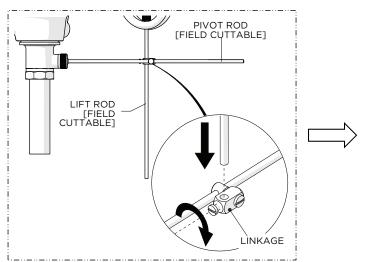
22. Connect the LIFT ROD to the PIVOT ROD using the LINKAGE provided.
