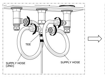
16. Connect the SIDEBODIES to the TEE using the SUPPLY HOSES provided. Securely tighten the HOSES and ensure they are not pinched/kinked.
