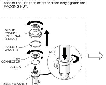
10. Unthread and remove the GLAND COVER, RUBBER WASHER, TRIM CONNECTOR and O-RING from the SIDEBODY then fully thread the NUT down the SIDEBODY.
