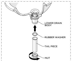
Re-attach the TAILPIECE then securely tighten the NUT onto the LOWER DRAIN BODY making sure to include the RUBBER WASHER provided.
