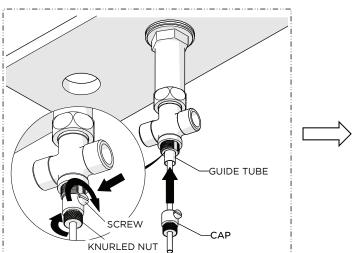
8. Slide the CAP up the LIFT ROD and onto the GUIDE TUBE then securely tighten the SCREW.
