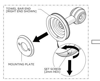
3. Loosen, but do <u>NOT</u> remove, the SET SCREW on the bottom of each TOWEL BAR END using a 2mm HEX KEY and remove the MOUNTING PLATES.
