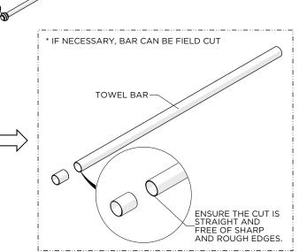
**OPTIONAL:** If necessary, the BAR may be cut. Ensure the cut is straight and free of sharp and rough edges.
