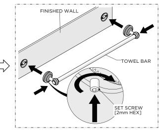
5. Holding the ENDS and BAR together, place both ENDS over the MOUNTING PLATES and securely tighten the SET SCREWS.
