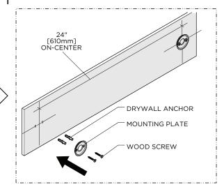
4. Using the previous marks as a reference, install the MOUNTING PLATES using the SCREWS and ANCHORS provided.
