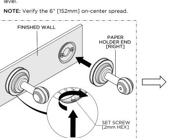
Place both PAPER HOLDER ENDS over the MOUNTING PLATES and securely tighten the SET SCREWS using a 2mm HEX KEY.
