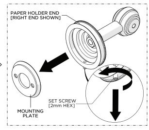
Loosen, but do <u>NOT</u> remove, the SET SCREW on the bottom of each PAPER HOLDER END using a 2mm HEX KEY and remove the MOUNTING PLATES.
