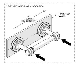
Dry-fit the product to the finished wall and mark the ideal location making sure to hold the product level.
