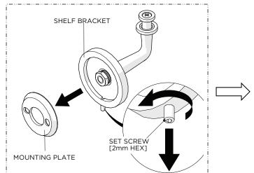
Loosen, but do <u>NOT</u> remove, the SET SCREW on the bottom of each SHELF BRACKET using a 2mm HEX KEY and remove the MOUNTING PLATES.
