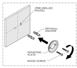
3. Using the previous marks as a reference, install the MOUNTING PLATE using the SCREWS and ANCHORS provided.
