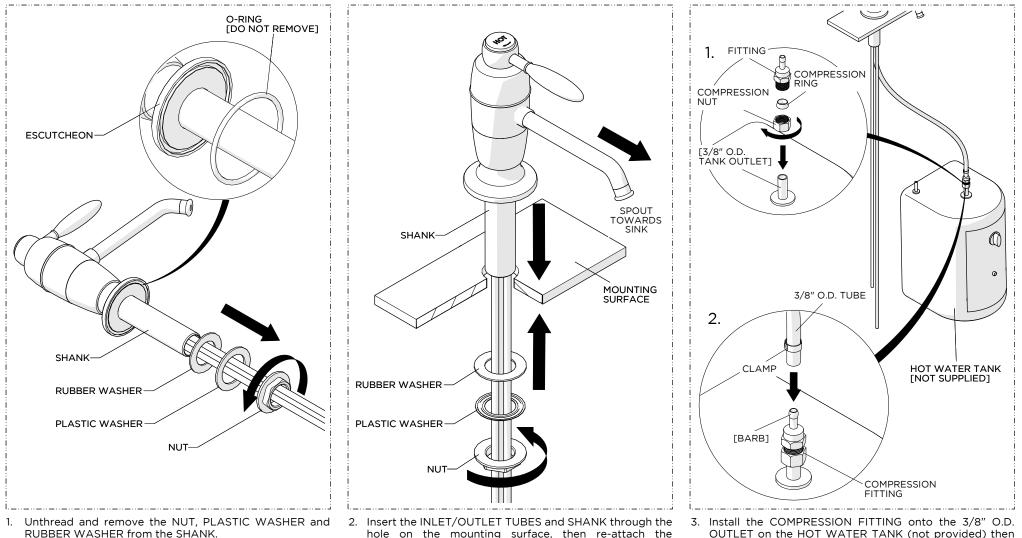
NOTE: Do NOT remove the O-RING beneath the ESCUTCHEON.
