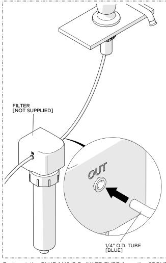
3. Insert the BLUE 1/4" O.D. INLET TUBE from the SPOUT into the WATER FILTER OUTLET (not supplied).
