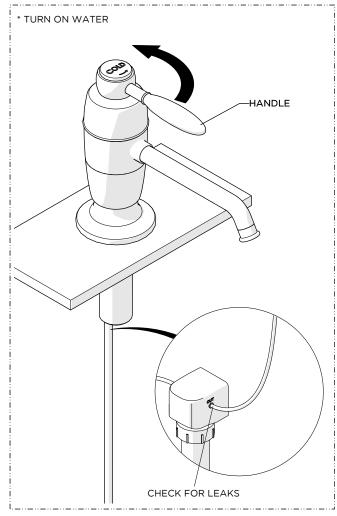
4. Turn on the water to flush out any debris in the supply line, operate the HANDLE and SPOUT to ensure they function properly and inspect all connections for leaks.
