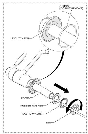
1. Unthread and remove the NUT, PLASTIC WASHER and RUBBER WASHER from the SHANK.
