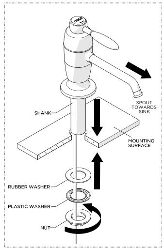
2. Insert the INLET TUBE and SHANK through the hole on the mounting surface, then re-attach the WASHERS and securely tighten the NUT.
