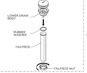
11. Remove the TAILPIECE from the LOWER DRAIN BODY.
