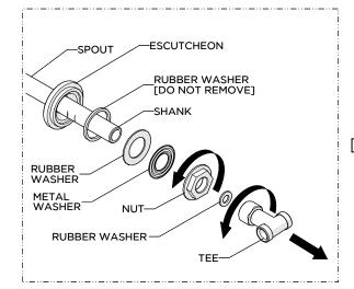
Remove the TEE, NUT and lower deck WASHERS from the SPOUT.
