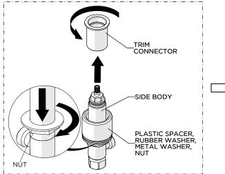
4. Unthread and remove the TRIM CONNECTOR then fully thread the NUT down the SIDEBODY.
