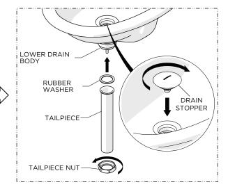
15. Re-install the DRAIN STOPPER then the TAILPIECE using the WASHER and NUT provided.
