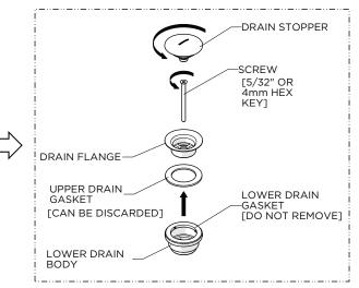
12. Unthread and remove the DRAIN STOPPER and LOWER DRAIN BODY from the DRAIN FLANGE The UPPER DRAIN GASKET can be discarded.
