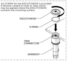
6. Making sure the O-RING is beneath the ESCUTCHEON, thread and securely tighten the ESCUTCHEON onto the TRIM CONNECTOR
