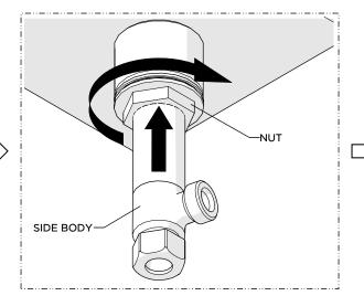
8. Ensure the HANDLE is properly aligned then securely tighten the NUT.
