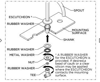
2. Insert the SPOUT through the hole on the mounting surface making sure the RUBBER WASHER provided is beneath the ESCUTCHEON then reinstall the WASHERS and NUT. Ensure the SPOUT is properly aligned then securely the NUT.
