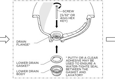
14. Re-install the LOWER DRAIN BODY making sure to use the GASKET provided. Ensure the GASKET makes a full seal on the underside of the lavatory then securely tighten the SCREW.
