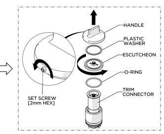
3. Loosen, but do **NOT** remove, the SET SCREW and remove the HANDLE then unthread and remove the ESCUTCHEON.
