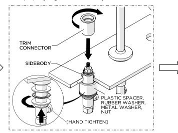
5. Thread the TRIM CONNECTOR back onto the SIDEBODY until it stops and let it rest on the mounting surface then hand-tighten the NUT against the underside of the mounting surface.
