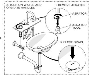
17. Removed the AERATOR, turn on the water to flush out the supply lines, and inspect all connections for leaks. Close the DRAIN.to ensure it functions properly then turn off the water and re-install the AERATOR.
