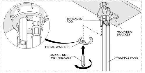
Slide the MOUNTING BRACKET over the HOSES and THREADED ROD, place the METAL WASHER onto the ROD, then thread and securely tighten the BARREL NUT onto the ROD.
