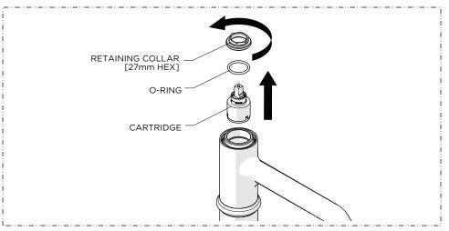
2. Unthread and remove the RETAINING COLLAR and O-RING then remove the CARTRIDGE.
