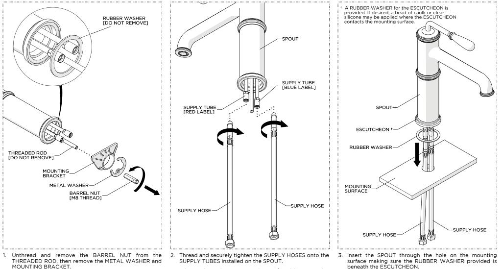
NOTE: Do NOT remove THREADED ROD or RUBBER WASHER beneath the ESCUTCHEON.
