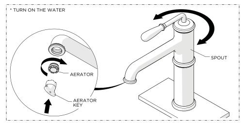
7. Re-install the AERATOR then turn on the water and operate the SPOUT to ensure it functions properly.
