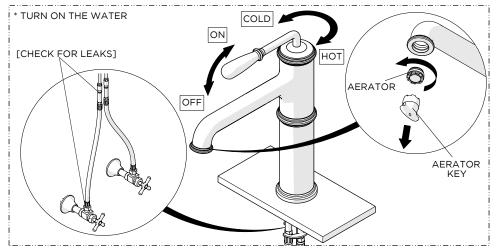
6. Unthread and remove the AERATOR from the SPOUT using the KEY provided. Turn on the water and operate the HANDLE to ensure it functions properly and flush out any debris in the supply lines then check all connections for leaks and turn off the water.
