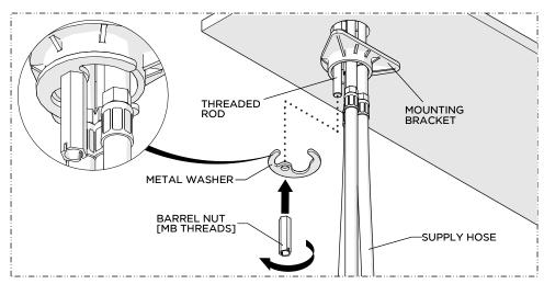
Slide the MOUNTING BRACKET over the HOSES and THREADED ROD, place the METAL WASHER onto the ROD, then thread and securely tighten the BARREL NUT onto the ROD.
