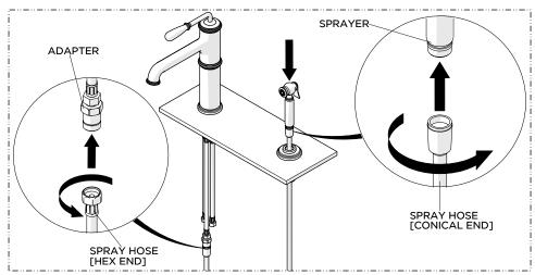
8. Thread and securely tighten the SPRAY HOSE (conical end) onto the SPRAYER and insert the HOSE into the PLASTIC SLEEVE until it stops then thread and securely tighten the HOSE (hex end) onto the ADAPTER.
