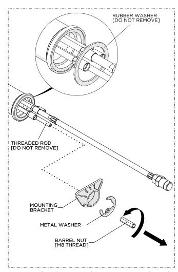
Unthread and remove the BARREL NUT from the THREADED ROD then remove the METAL WASHER and MOUNTING BRACKET.
