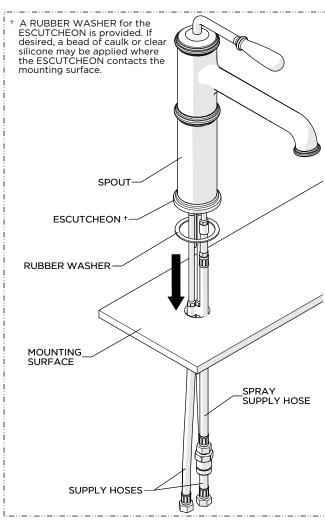
Insert the SPOUT through the hole on the mounting surface making sure the RUBBER WASHER provided is beneath the ESCUTCHEON.
