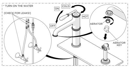
10. Unthread and remove the AERATOR from the SPOUT using the KEY provided. Turn on the water and operate the HANDLE to ensure it functions properly and to flush out any debris in the supply lines then check all connections for leaks and turn off the water.
