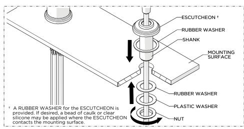
7. Insert the SHANK through the hole on the mounting surface making sure the RUBBER WASHER is beneath the ESCUTCHEON. Re-install the WASHERS then thread and securely tighten the NUT.
