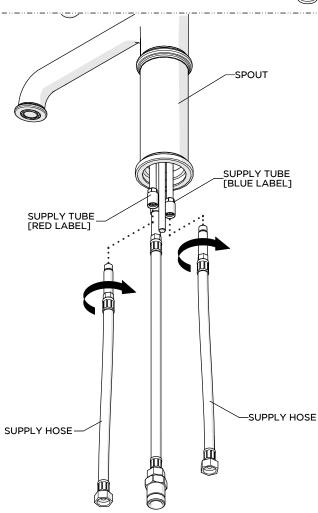
2. Thread and securely tighten the SUPPLY HOSES onto the SUPPLY TUBES installed on the SPOUT.
