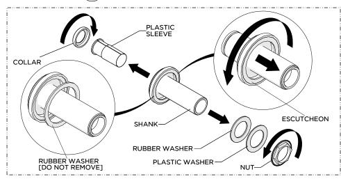
5. Unthread and remove the COLLAR, PLASTIC SLEEVE, NUT and WASHERS from the SHANK, then partially unthread the ESCUTCHEON.
