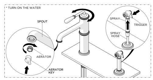
11. Re-install the AERATOR then turn on the water and operate the SPRAY and SPOUT to ensure they function properly.
