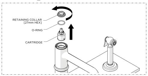
Unthread and remove the RETAINING COLLAR and O-RING then remove the CARTRIDGE.
