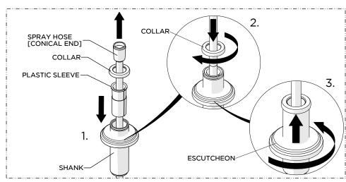
6. Insert the SPRAY HOSE (conical end) through the SHANK, PLASTIC SLEEVE and COLLAR then insert the SLEEVE back into the SHANK. Thread and securely tighten the COLLAR onto the SHANK then thread the ESCUTCHEON up until it stops.
