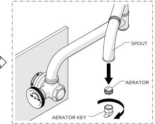
6. Unthread and remove the AERATOR from the SPOUT using the AERATOR KEY provided.
