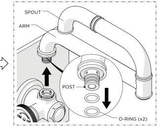
2. Remove the ARM to expose the POST and access the O-RINGS.
