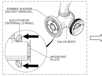
1. Slide the ESCUTCHEON against the VALVE BODY to expose the SET SCREWS.
