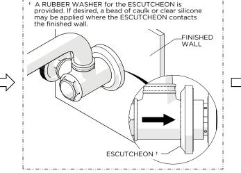
8. Slide the ESCUTCHEON down the VALVE BODY until it contacts the finished wall.
