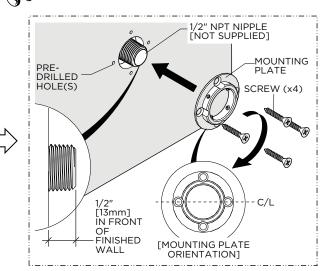
3. Ensure the NIPPLE (not supplied) protrudes 1/2" [13mm] in front of the finished wall then install the MOUNTING PLATE, in the proper orientation, using the SCREWS (x4) provided.
