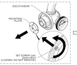
2. Loosen, but do **NOT** remove, the SET SCREWS (x4) using a 2mm HEX KEY then remove the MOUNTING PLATE from the VALVE BODY.
