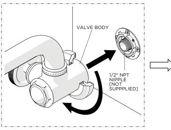
4. Thread and securely tighten the VALVE BODY onto the NIPPLE (not supplied).
