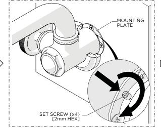
5. Securely tighten the SET SCREWS (x4) on the MOUNTING PLATE using a 2mm HEX KEY to secure the SPOUT and prevent it from rotating.
