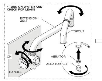
7. Turn on the water and operate the HANDLE to flush out any debris in the supply line and check for leaks then turn off water and re-install the AERATOR.
