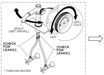
7. Turn on the water and operate the HANDLE and SPOUT to ensure they function properly and to flush out any debris in the supply lines then check all connections for leaks and turn off the water.
