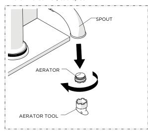
6. Using the tool provided, remove the AERATOR.
