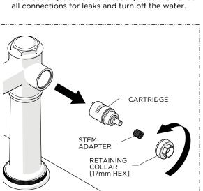
2. Unthread and remove the RETAINING COLLAR to expose the CARTRIDGE and STEM ADAPTER.
