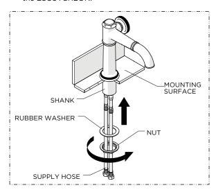
Slide the RUBBER WASHER and NUT over the SUPPLY HOSES and TUBES then, making sure the HANDLE is properly aligned, thread and securely tighten the NUT.
