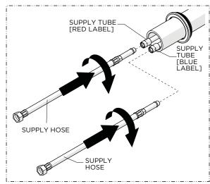
Thread and securely tighten the SUPPLY HOSES onto the SUPPLY TUBES installed on the SPOUT.
