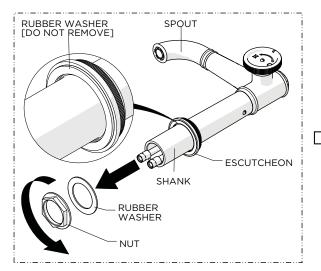
Remove the NUT and RUBBER WASHER from the SPOUT SHANK.
