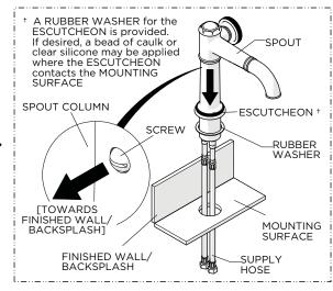
Insert the SPOUT through the hole on the mounting surface making sure the RUBBER WASHER provided is beneath the ESCUTCHEON and the SCREW on the SPOUT CLOUMN is aligned towards the finished wall/backsplash.
