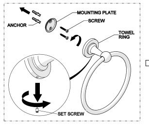
1. Unthread the SET SCREW and remove the MOUNTING PLATE, SCREWS and ANCHORS from TOWEL RING.
