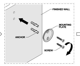
2. Secure the MOUNTING PLATE onto the finished wall using the SCREWS provided.
