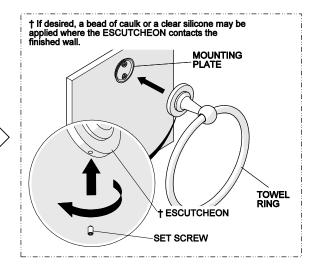
3. Place the TOWEL RING over the MOUNTING PLATE then thread and securely tighten the SET SCREW into the ESCUTCHEON.
